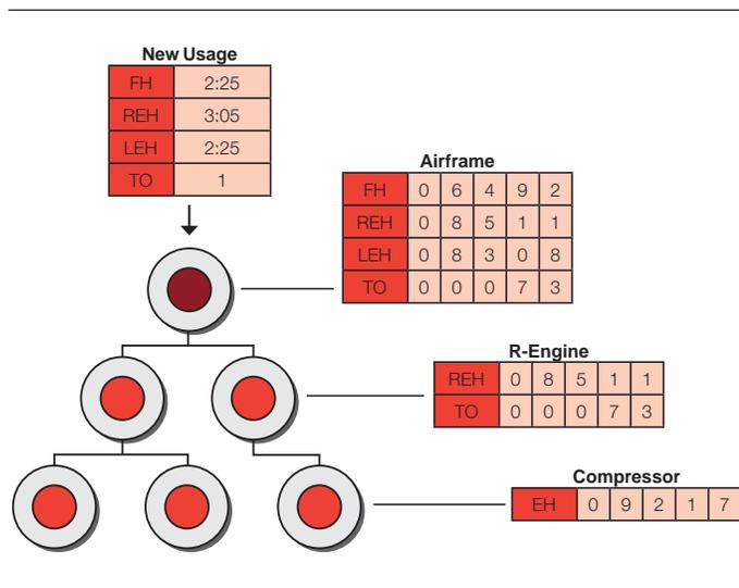
Figure 1: Conventional component life tracking, using cumulative transactions
