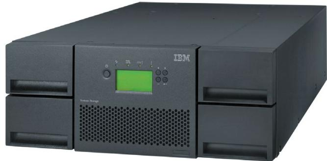
TS3200 Tape Library, featuring full- and half-height technology, offers 8 Gbps Fibre Channel for LTO Ultrium 8, 7, 6 and 5, and 6 Gbps SAS interfaces for LTO Ultrium 8, 7, 6 and 5. It can be attached to a wide variety of open-system servers. The sequential or random-access library comes in a standalone or optional rack-mountable configuration. TS3200 Tape Library also has an LCD display and indicators for power, drive and activity, error status, and message information.
