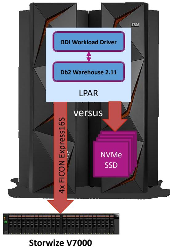
Figure 6: Db2 benchmark configuration showing Storwize V7000 and NVMe attachment
