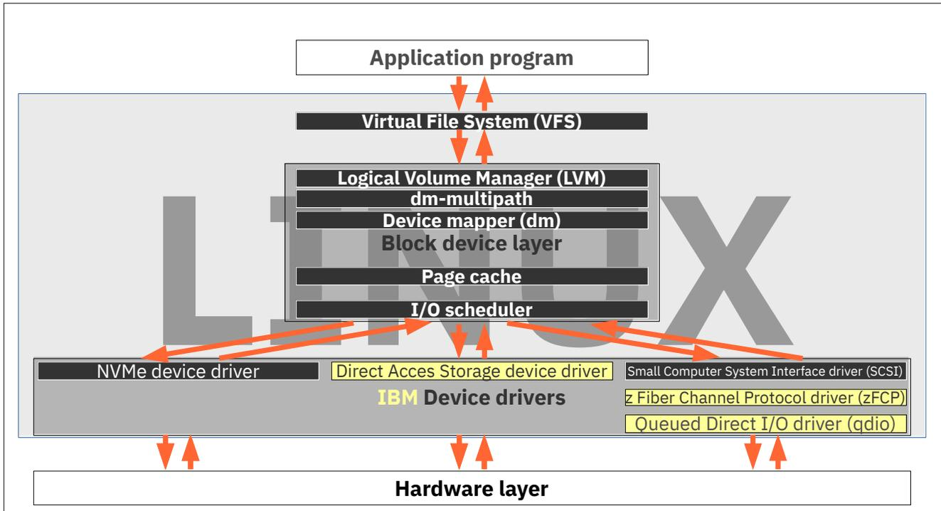
Figure 1: Overview of Linux disk I/O flow
