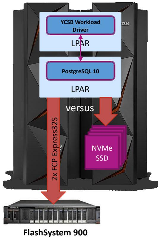
Figure 5: Postgre benchmark configuration showing FlashSystem and NVMe attachment
