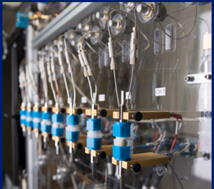
Battery tester and cycler at IBM Research
