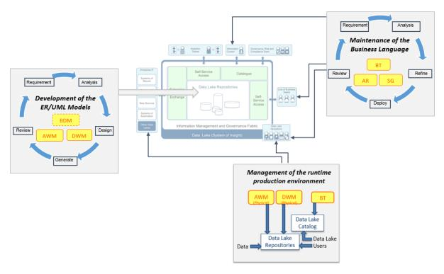
The diagram above shows the three different lifecycles, the different IBM Industry Model components that they would typically be expected to evolve and manage and where these lifecycles would typically connect with the data lake Landscape.
