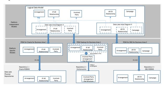
In the diagram above the Logical Data Model has a single set of actual entities (for example, Arrangement, Involved Party, etc), with each of the diagrams having read-only views of these entities. It is assumed that in each entity the specific subset of attributes that would be persisted are indicated using the IDA Persistence flag for that attribute. The setting of such a persistence flag is cumulative (all the attributes needed for all diagrams are set as "persisted" in the actual entity).
