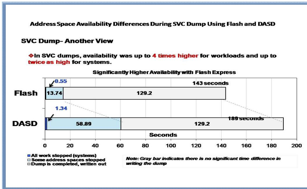
Figure 4. SVC Dump comparison chart showing non dispatchable time
