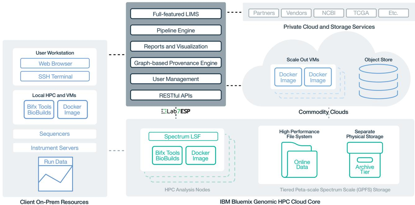
Figure 1: Architecture of the Lab7 High-Performance Genomic Cloud, running on the IBM Bluemix cloud platform
