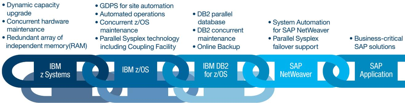
Figure 2: Together, these components form a highly available business continuity solution for SAP on IBM z Systems.
