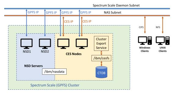
Our test setup is comprised of four Spectrum Scale nodes — two NSD servers and two CES nodes.
