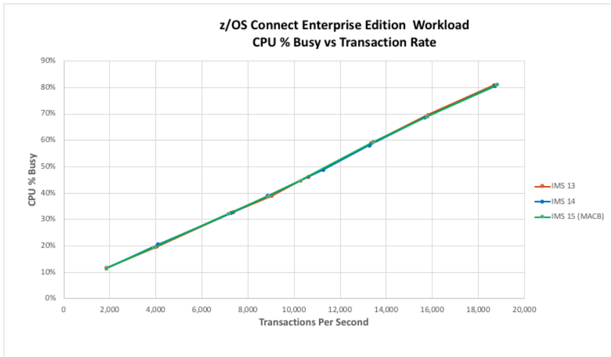
Figure 38: z/OS Connect EE SP CPU % Busy vs Transaction Rate Comparison
