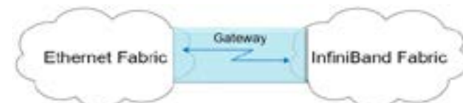
Figure 3: InfiniBand to Ethernet Gateway
