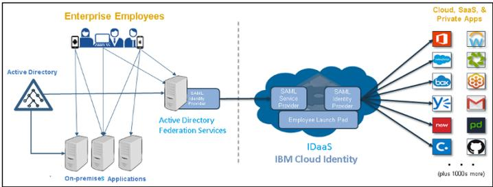
**FIGURE 3-1:** Accessing on-premises and SaaS applications with IDaaS.
