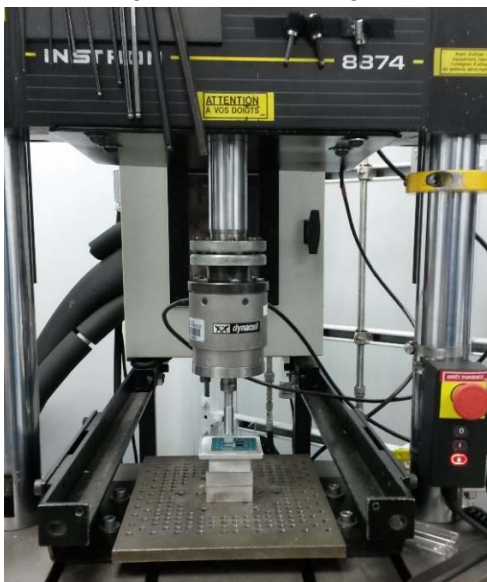
Figure 4. Instron 8874 use for compressive tests.
