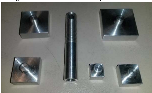
Figure 5. The five pressure heads and the shaft used in the compressive load tests.
