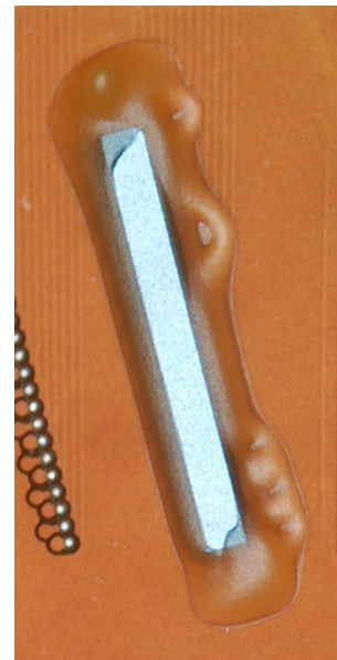
Figure 7. Sidefill material is dispensed around the OE chip. Assembly yield improvement by the sidefill process has been confirmed.
