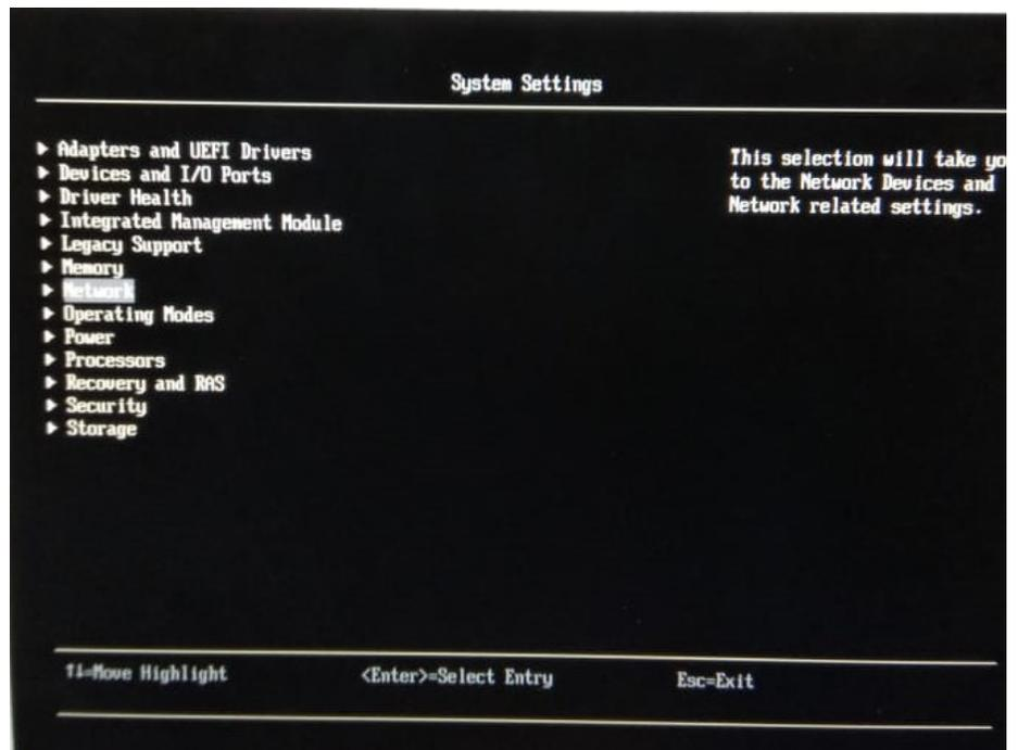
5. On the Network page, the network devices are displayed. In the list, verify the Cavium adapter ports. The ports will be listed if it is detected by BIOS. In this example, you can see that two ports are listed. Older BIOS would not list the Cavium adapter ports.
