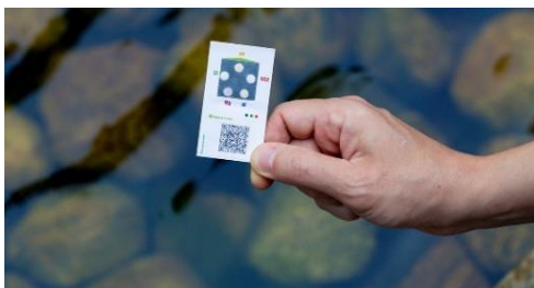
The AgroPad - a set of circles on the back of the card provide colorimetric test results; the color of each circle represents the amount of a particular chemical in the sample.
