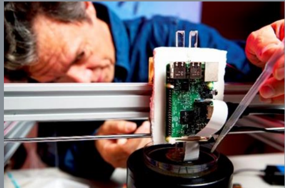
IBM researcher, Tom Zimmerman, evaluates a seagoing microscope which will be used to analyze plankton.
