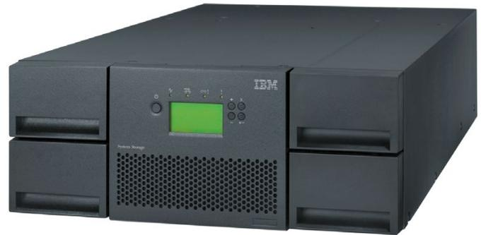
TS3200 Tape Library, featuring full- and half-height technology, offers 8 Gbps Fibre Channel (FC) for LTO Ultrium 8, 7, 6 and 5 and 6 Gbps SAS interfaces for LTO Ultrium 8, 7, 6 and 5. It can be attached to a wide variety of open-system servers. The sequential or random-access library comes in a standalone or optional rack-mountable configuration. TS3200 Tape Library also has an LCD display and indicators for power, drive and activity, error status and message information.
