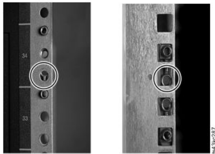
Figure 3. Correct connector locations
