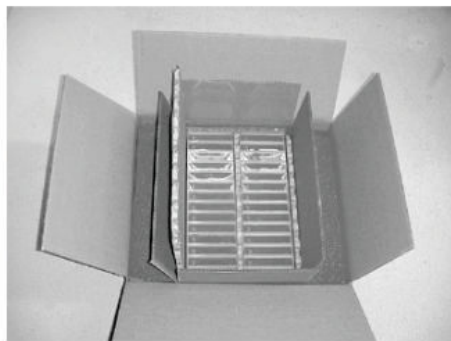
Figure 2. Double-boxing tape cartridges for shipping
