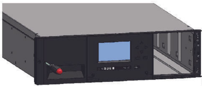
Figure 2. Manually releasing the left magazine
