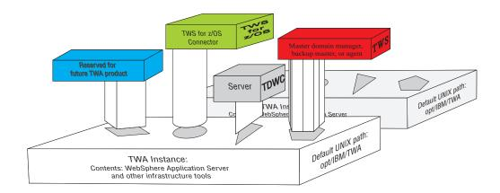
The above image shows two instances of Tivoli Workload Automation. A component of Tivoli Workload Scheduler, Dynamic Workload Console, and the Tivoli Workload Scheduler for z/OS connector are shown ready to be plugged in to the Tivoli Workload Automation instance. Each "Tivoli Workload Automation instance" contains an instance of the embedded WebSphere Application Server.
