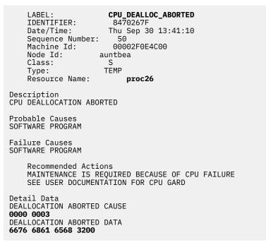
In this example, the deallocation for **proc26** failed. The reason code 3 means that a kernel extension returned an error to the kernel notification routine. The DEALLOCATION ABORTED DATA above spells **fvhaeh2**, which is the name the extension used when registering with the kernel.
