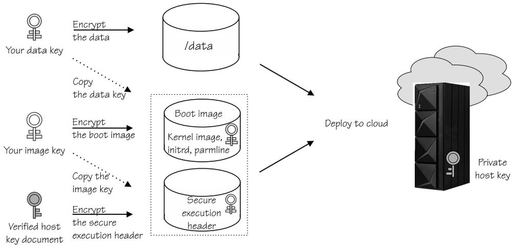
Figure 5. Conceptual key cascade for IBM Secure Execution
