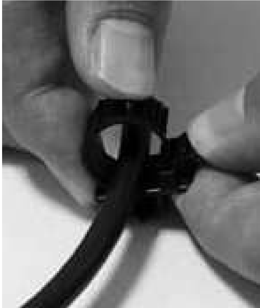
Figure 55. Unlocking the cable retention bracket
