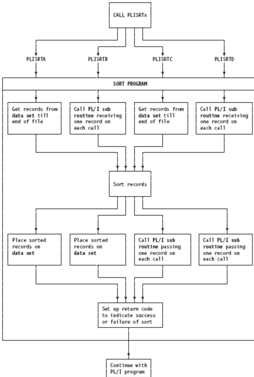
Figure 7. Flow of control for Sort program
