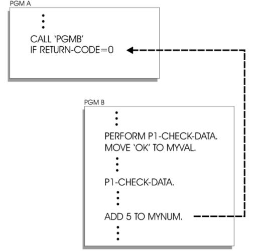
Assume that the current execution point is on PGM B and, at the line ADD 5 TO MYNUM. At this point, you decide you don't need to see any more of the code in PGM B. By issuing STEP RETURN on the command line, z/OS Debugger returns to the first line of code after the CALL command that called PGM B, as indicated by the arrow. You can then continue stepping through PGM A.
