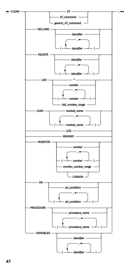
Removes all breakpoints, including GLOBAL breakpoints, set by previously entered AT commands, except for AT TERMINATION and suspended breakpoints.
