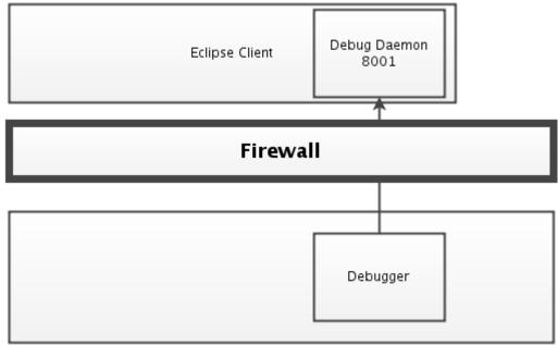
Figure 4. TCP/IP port for the usage of z/OS Debugger without Debug Manager
