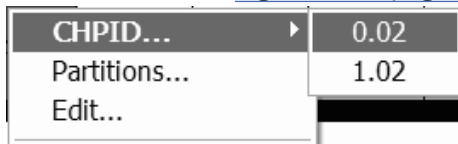
Figure 13. Context menu of a spanned CHPID in a vertical processor view
