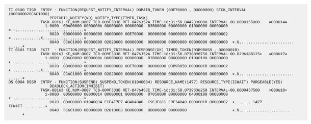
Figure 25. Trace entries showing interval calculation and task suspension
