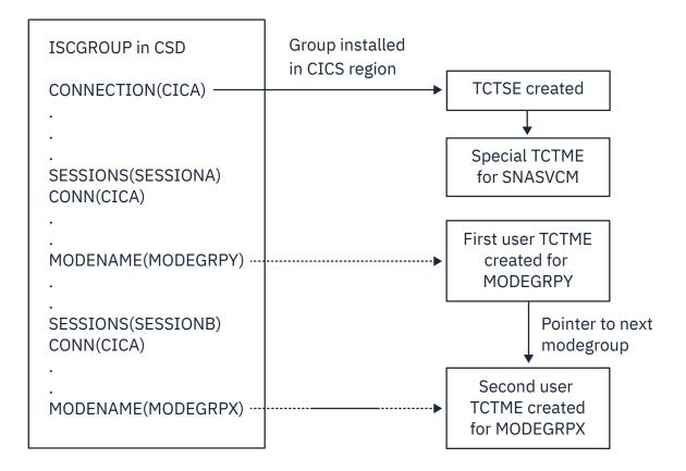
Figure 1. How the sequence of TCT mode entries is determined
