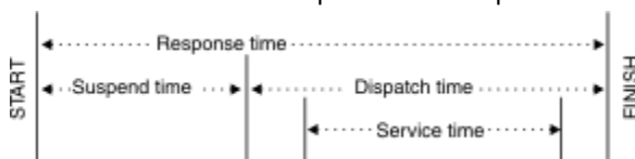
Figure 6. CICS internal response-time elements
