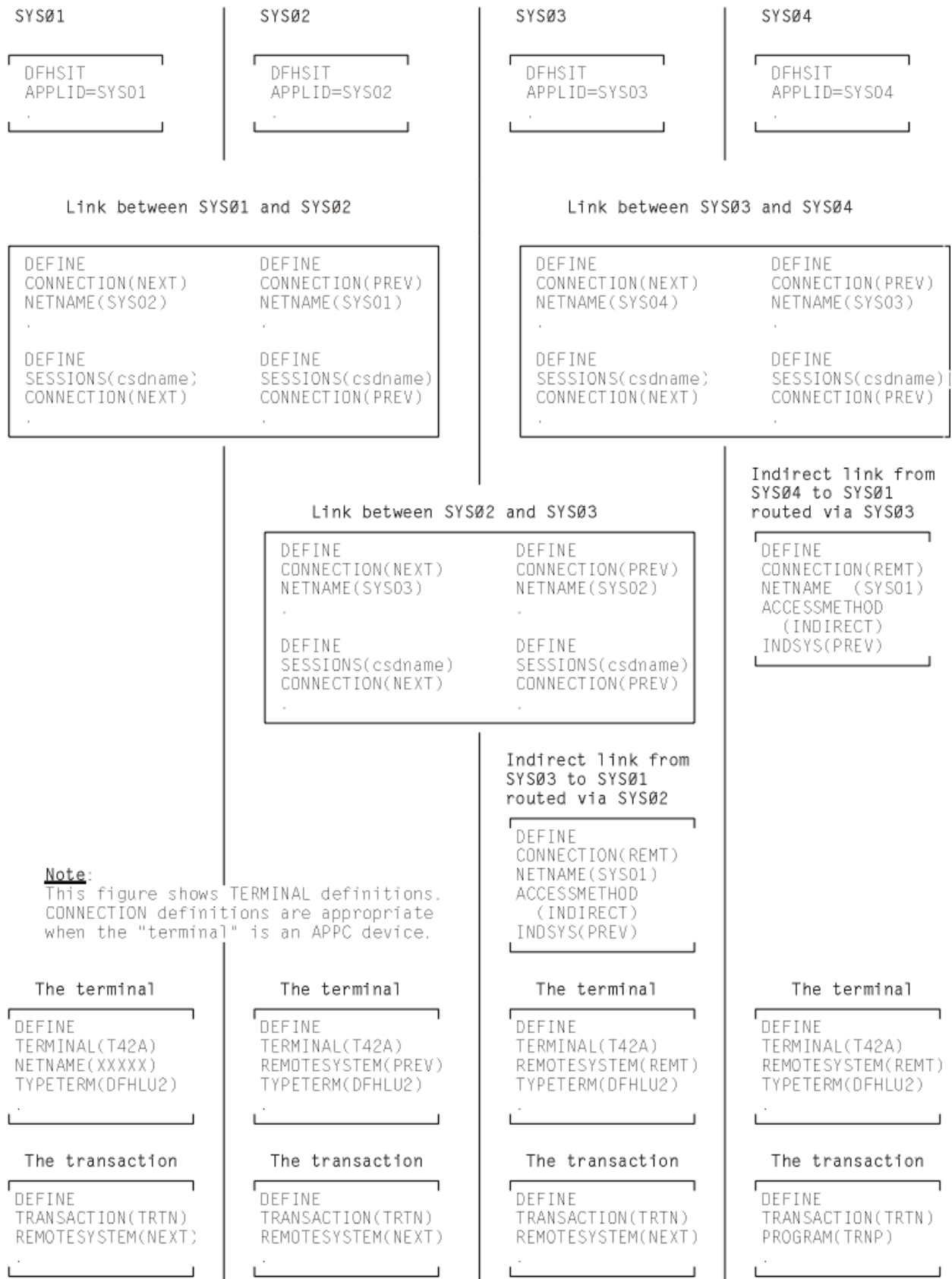
Figure 51. Defining indirect links for transaction routing
