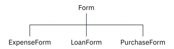
Each form needs printing at some time. In procedural programming, we would either code a print function to handle the three different forms or we would write three different functions (printExpenseForm, printLoanForm, printPurchaseForm).
