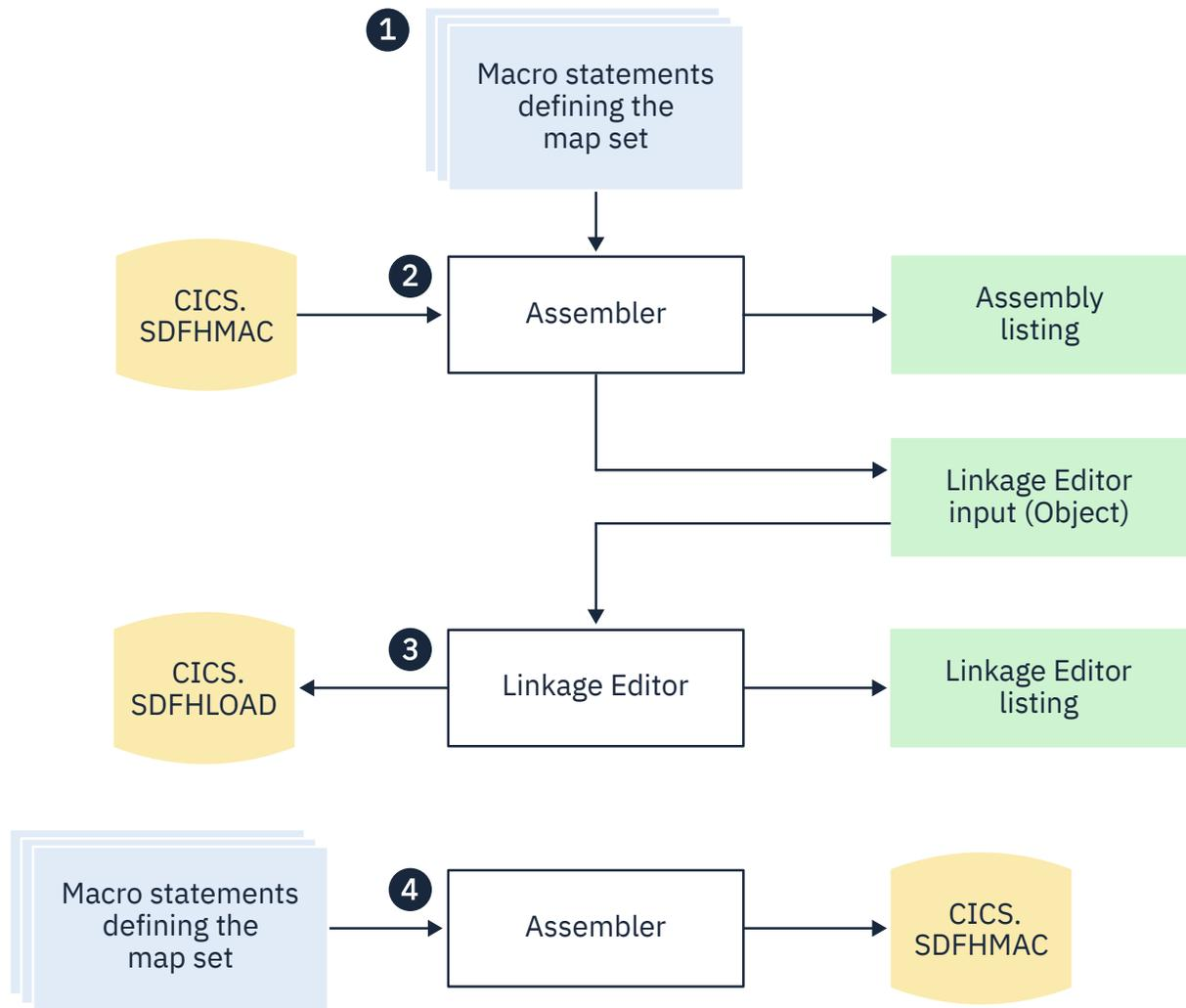
Figure 174. Installing a physical map set and a symbolic description map set together
