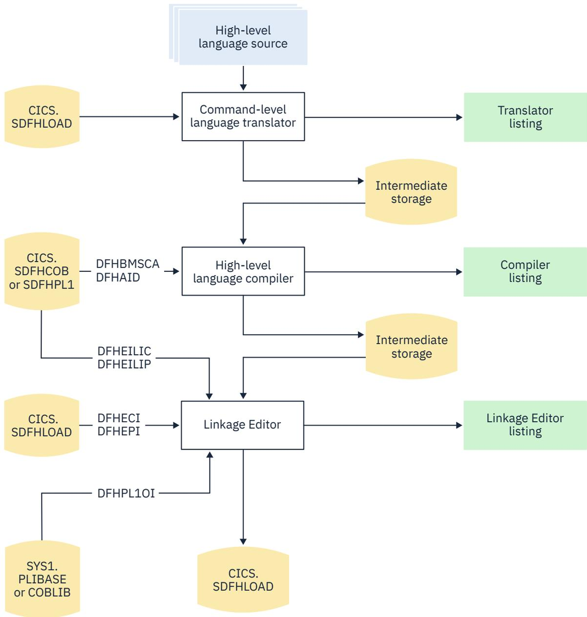
Figure 160. Installing COBOL and PL/I programs
