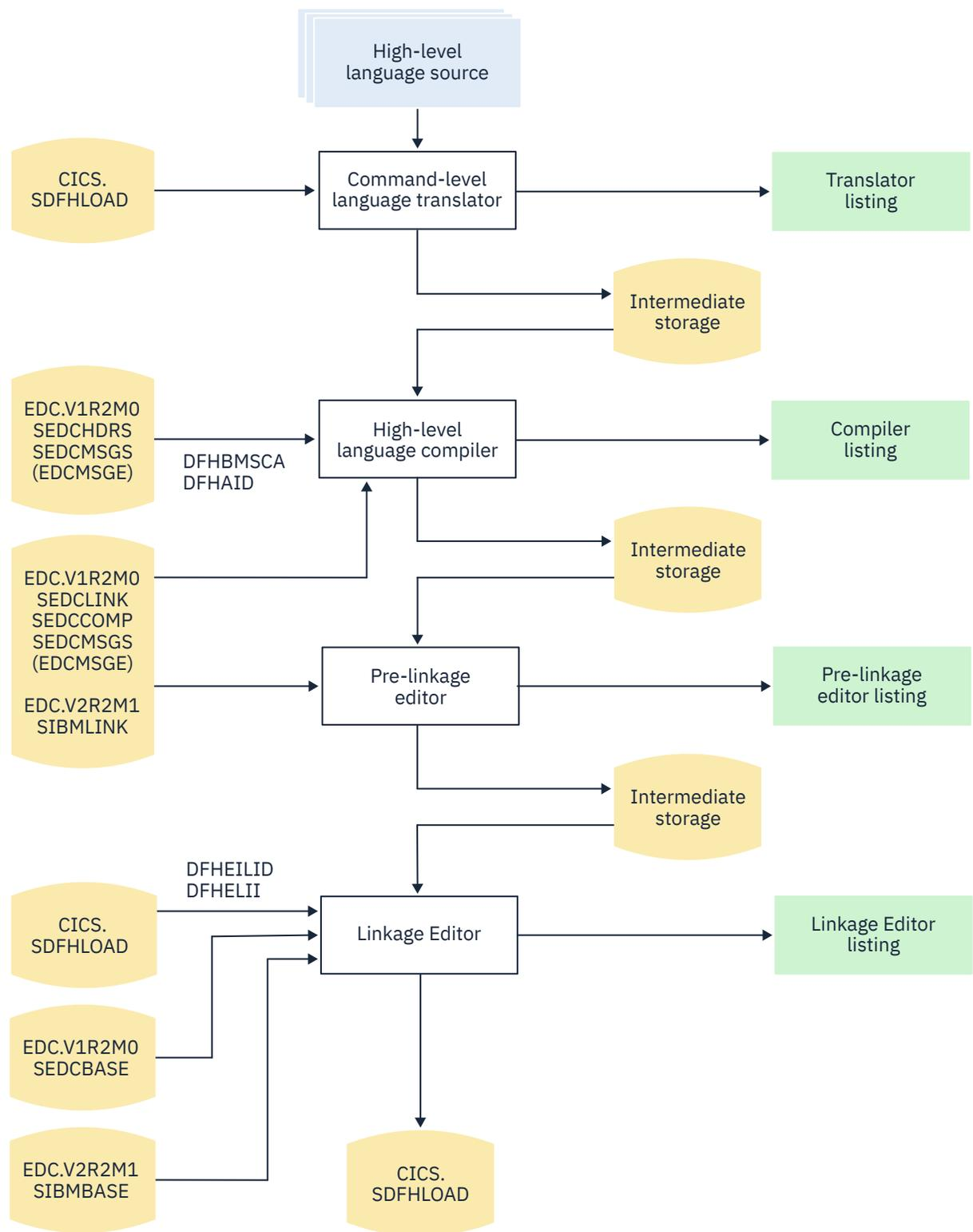
Figure 163. Installing C programs using the DFHYxTzL procedure
