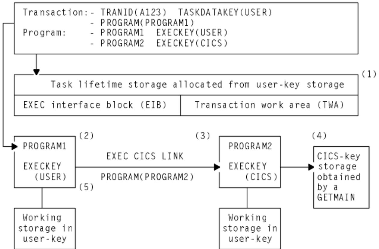
Figure 92. Illustration of the use of the TASKDATAKEY and EXECKEY options
