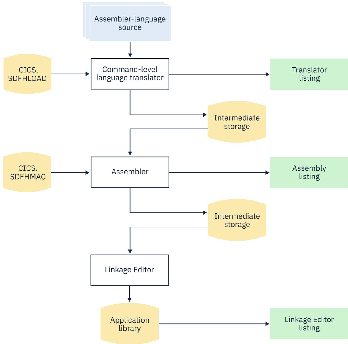
Figure 159. Installing assembler language programs using the DFHEITAL or DFHEGTAL procedure
