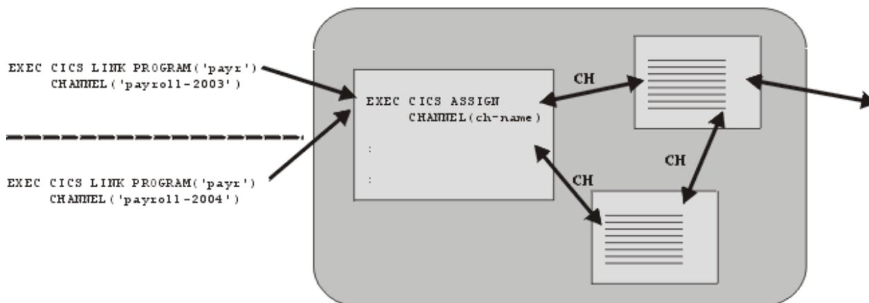
Figure 30. Multiple external channels to the same component
