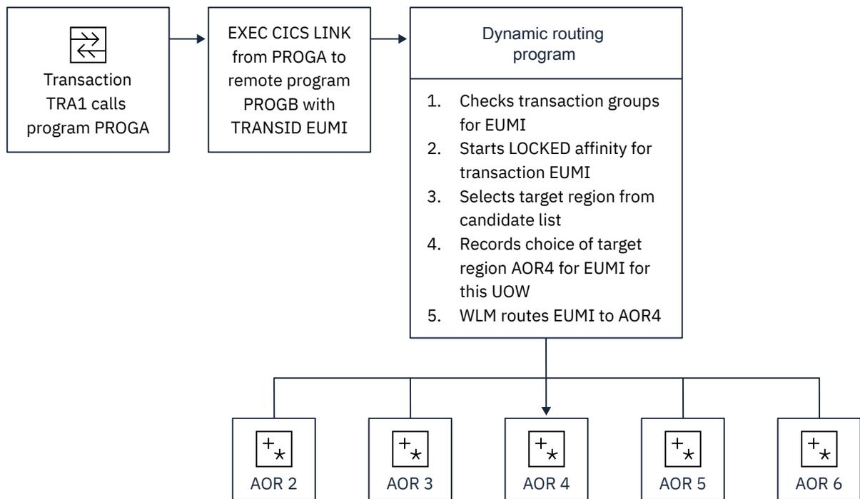
Figure 66. Managing inter-transaction affinity with LOCKED relation and UOW lifetime
