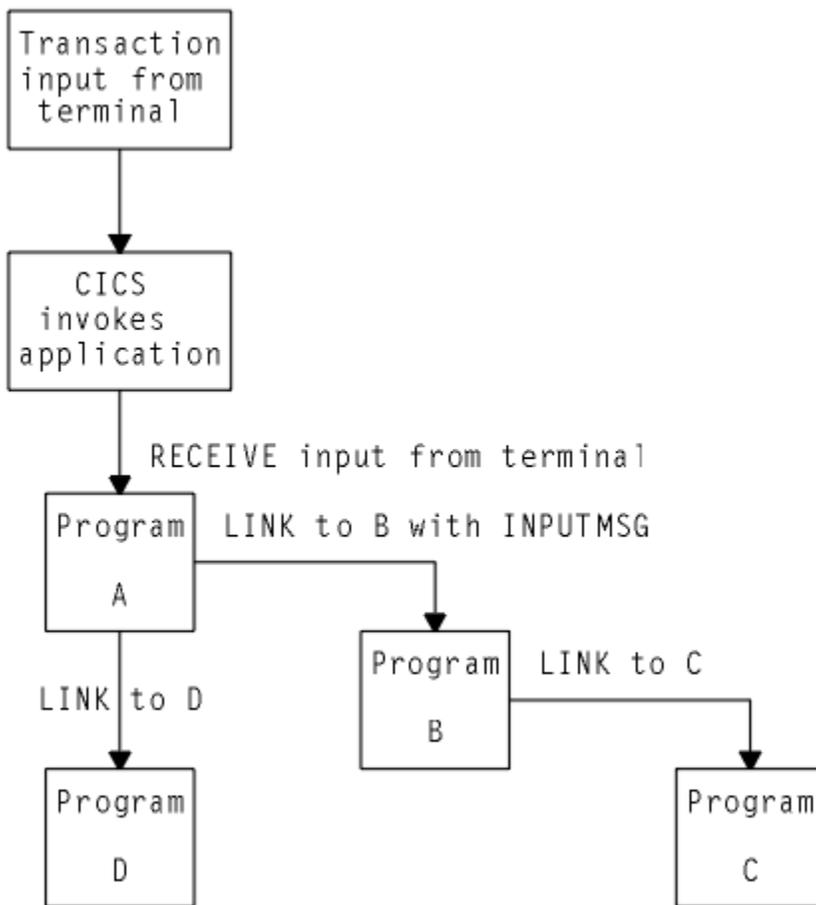
Figure 40. Use of INPUTMSG in a linked chain
