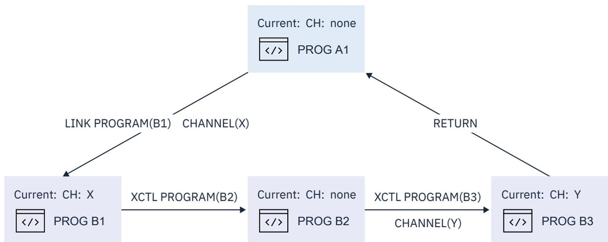
Figure 33. Current channels—example, with XCTL commands
