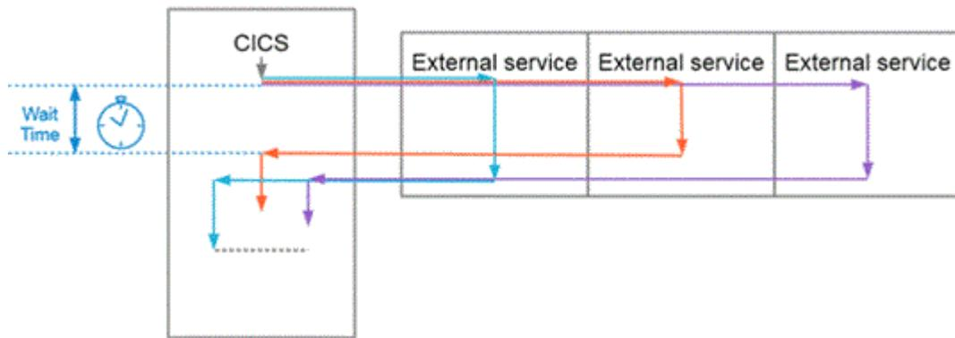
Figure 2. Calling services in parallel (asynchronous processing)
