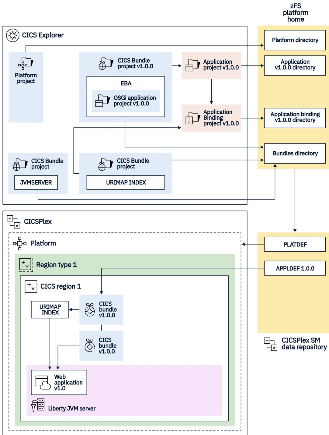
Figure 18. Example topology for Version 1.0.0 of the application
