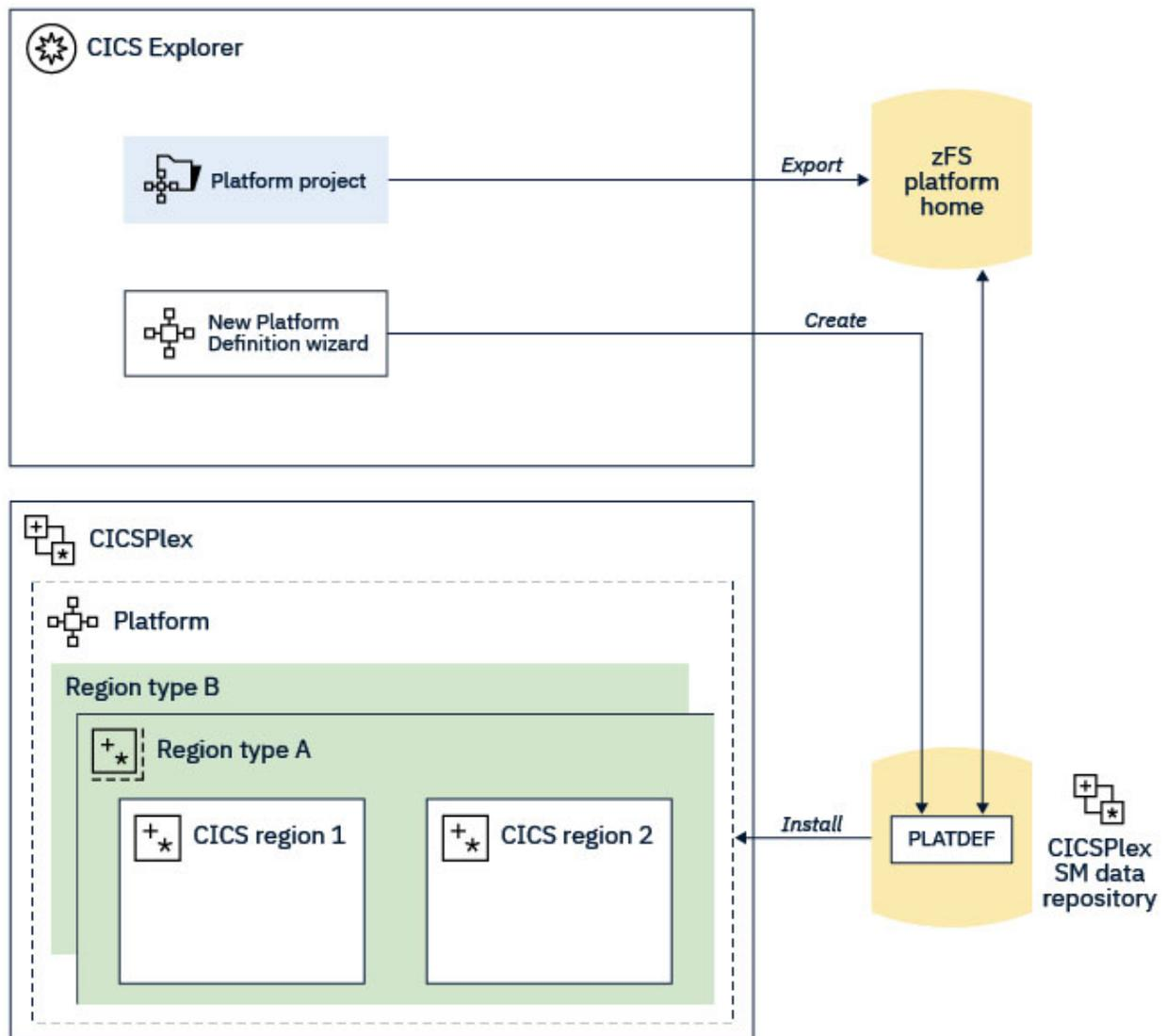
Figure 9. Creating the elements of a platform
