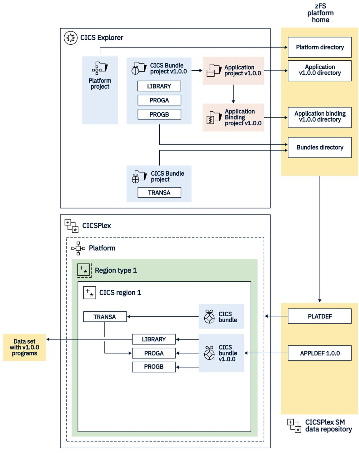
Figure 16. Example topology for Version 1.0.0 of the application
