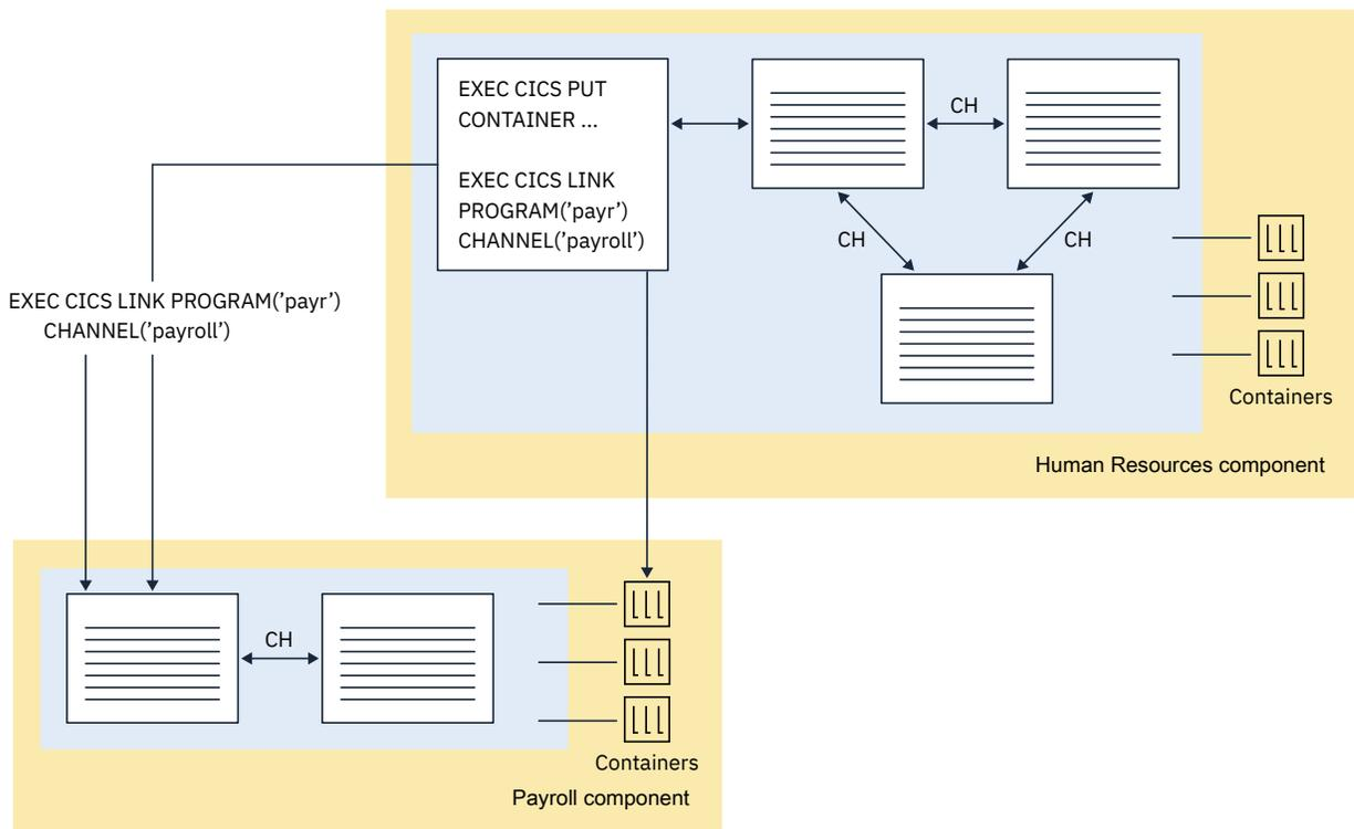
Figure 31. Multiple components which interact through their channels
