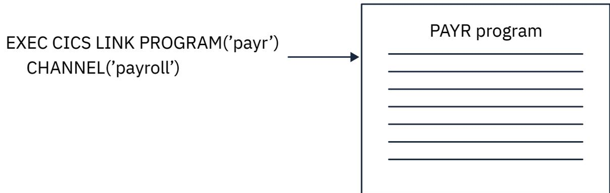
Figure 28. A stand-alone program with a single channel
