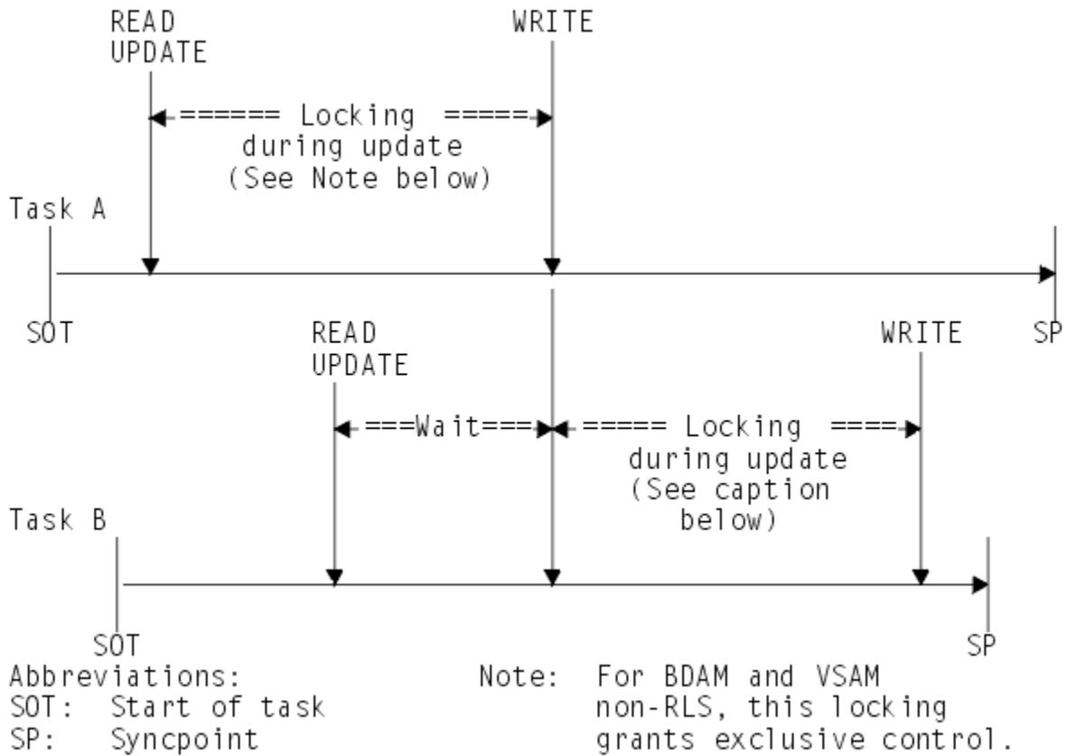
Figure 131. Locking during updates to nonrecoverable files
