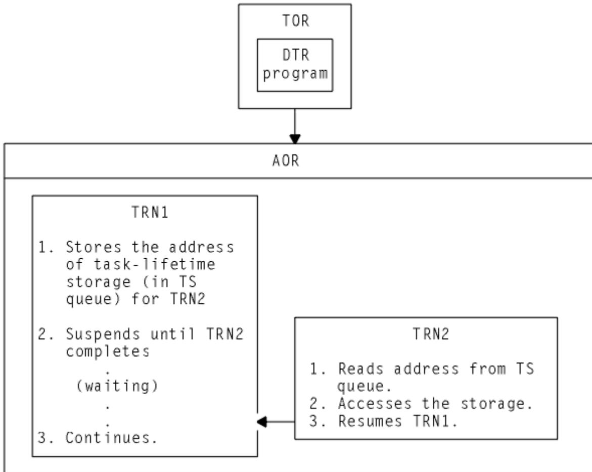
Figure 54. Illustration of inter-transaction affinity created by use of task-lifetime storage
