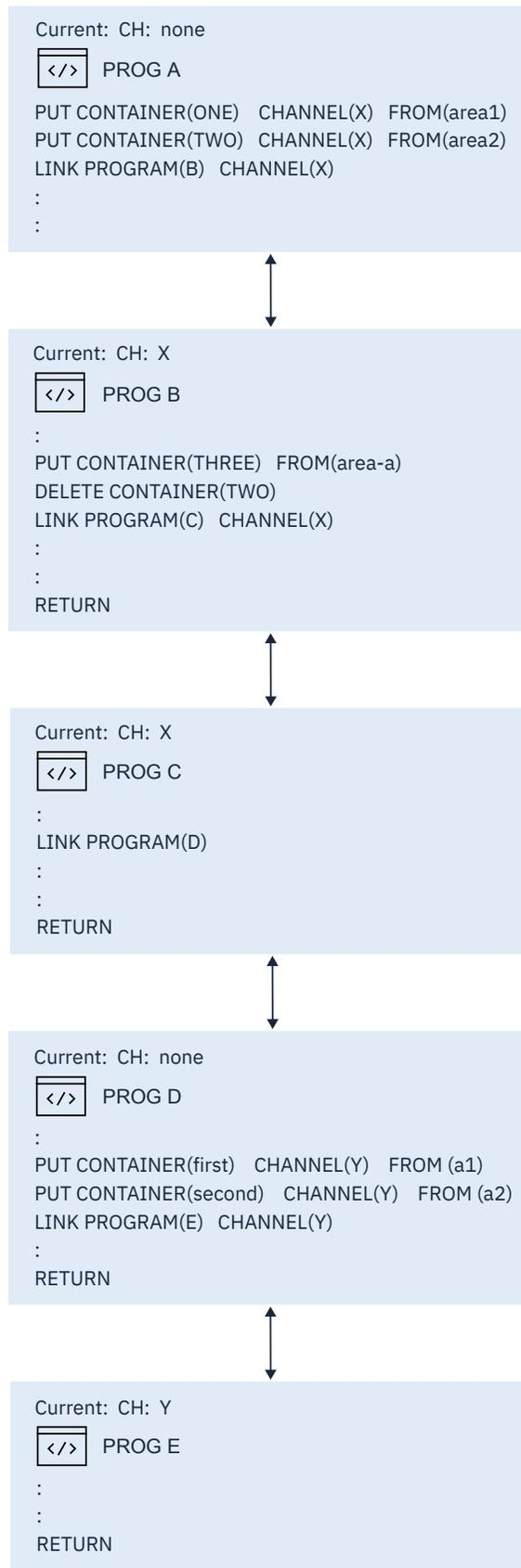
Figure 32. Current channel: example with LINK commands
