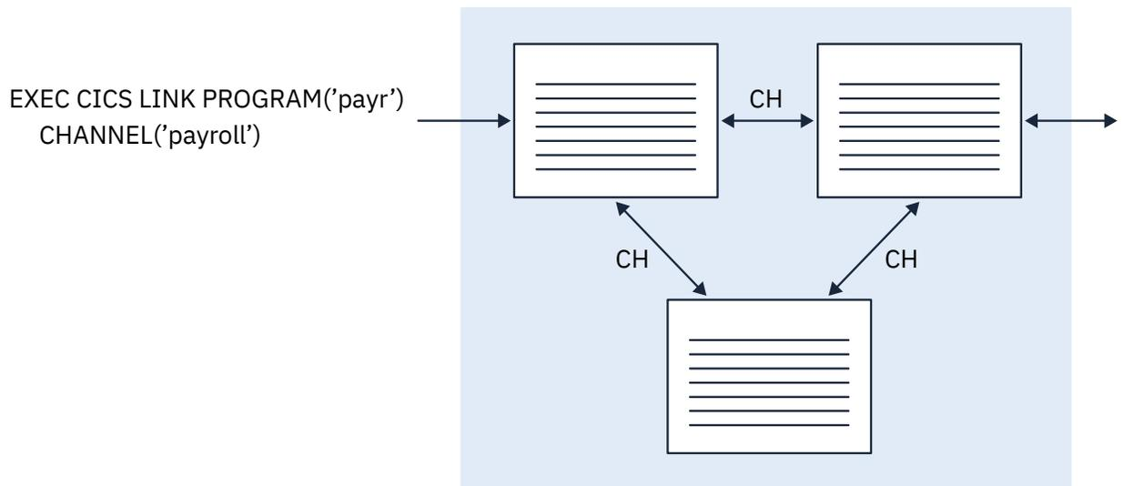
Figure 29. A "component" —a set of related programs invoked through a single external channel
