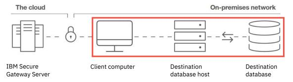
The ACL is a file in which you list the names and port numbers of computers that are permitted to host your on-premises data via the Secure Gateway.
