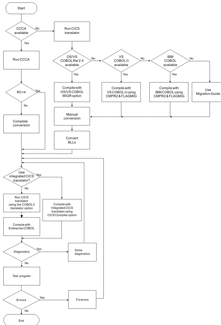
Figure 2. Steps for converting an OS/VS COBOL program containing CICS commands
