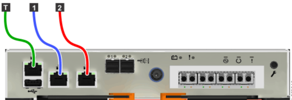
Figure 78. Connecting the Ethernet cables to a Storwize V5030E system
