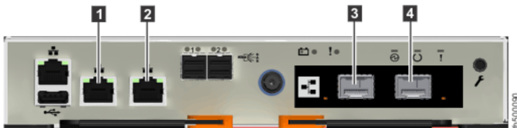
Figure 79. Example of a Storwize V5030E system with a 2-port Ethernet host interface adapter
