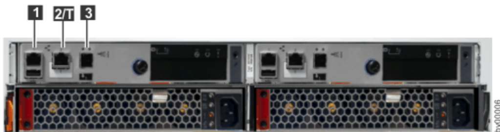
Figure 11. Data ports on the rear of the Storwize V5010E control enclosure
