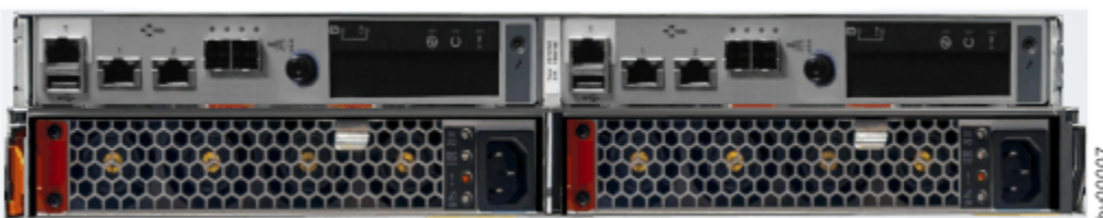
Figure 10. Storwize V5030E control enclosure
