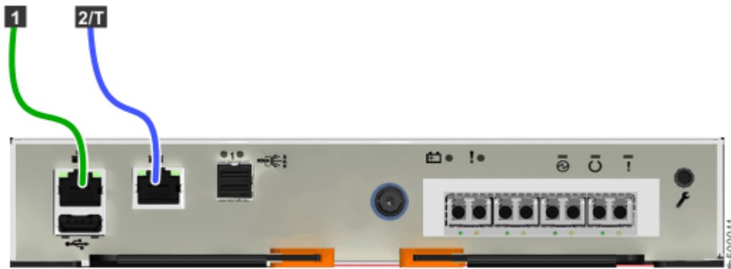
Figure 77. Connecting the Ethernet cables to a Storwize V5010E system
