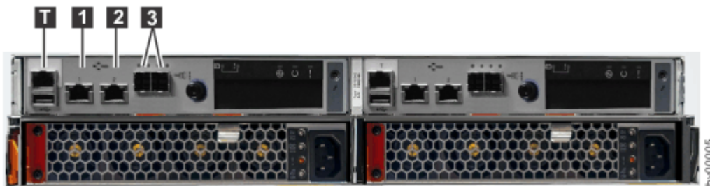
Figure 12. Data ports on the rear of the Storwize V5030E control enclosure
