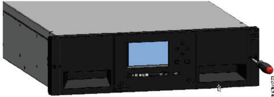
Figure 84. Manually releasing the right magazine
