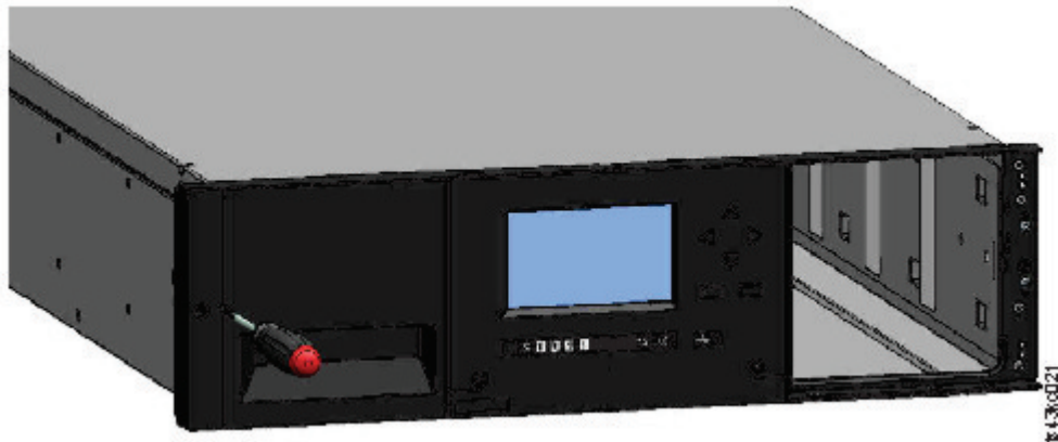
Figure 85. Manually releasing the left magazine
