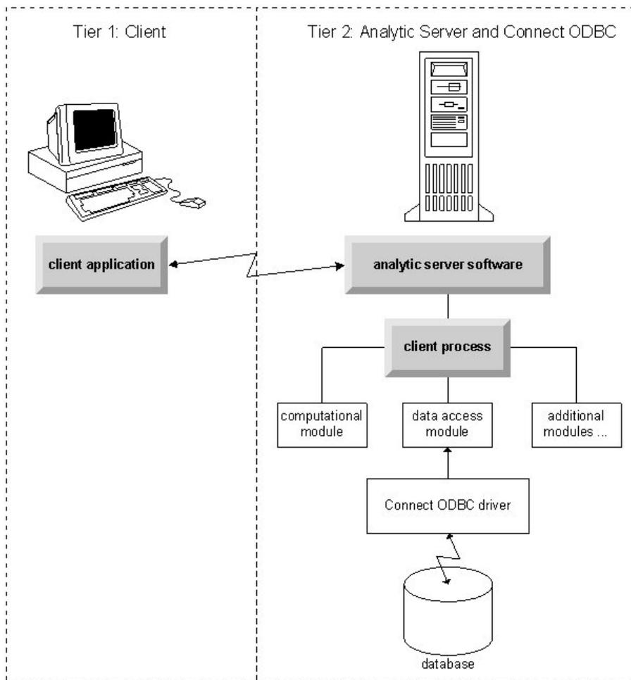
Figure 1. Connect ODBC in distributed analysis mode
