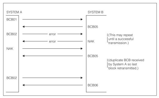
Figure 17. Correct Recovery with Null Records
