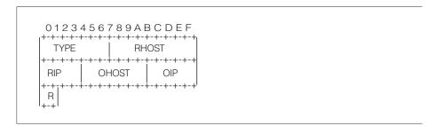
Figure 59. Format for the control record
