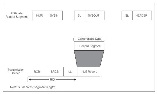
Figure 9. Format of a transmission buffer for SNA protocol
