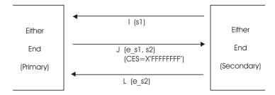
Figure 36. Secure connection (non-path manager trunk)
