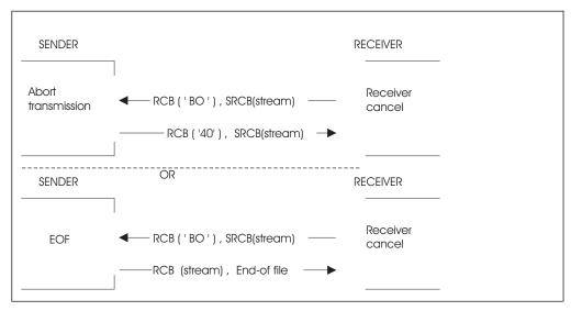
Figure 27. Receiving Node Initiates Stream End
