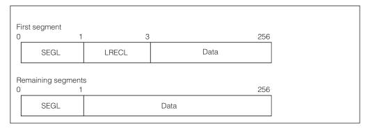
Figure 22. Spanned Data Record
