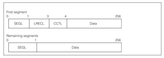
Figure 23. Spanned Data Record With Carriage Control
