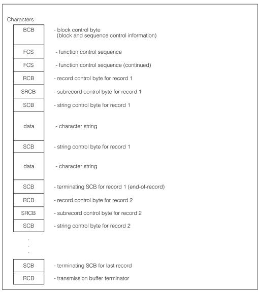
Figure 15. Format of a Transmission Buffer for BSC and CTC
