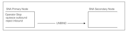
Figure 14. Terminating Processing by an SNA Primary Node
