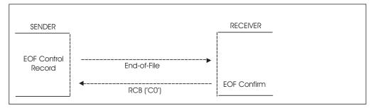
Figure 25. Protocols Used to Transmit a Stream
