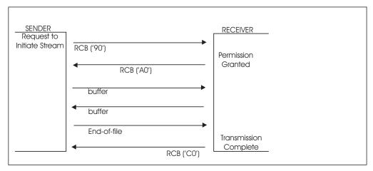
Figure 24. Protocols Used to Transmit a Stream
