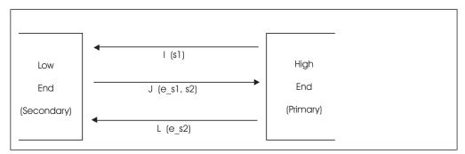
Figure 33. Secure connection (high initiates)
