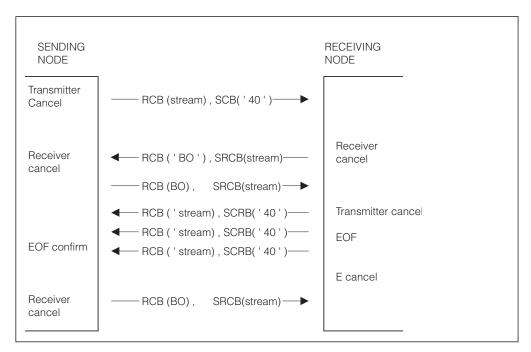
Figure 26. Sending Node Initiates Stream End
