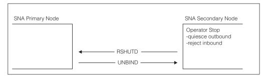
Figure 13. Terminating Processing by an SNA Secondary Node
