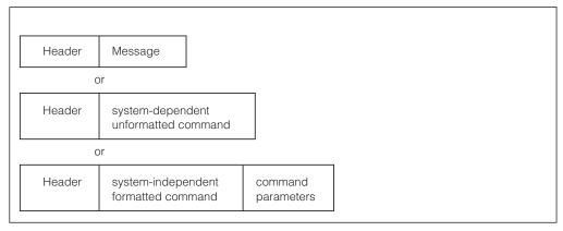
Figure 7. Format of an NMR
