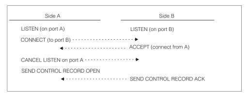
Figure 58. Description of new protocol allowing transfer of CTC NJE data
