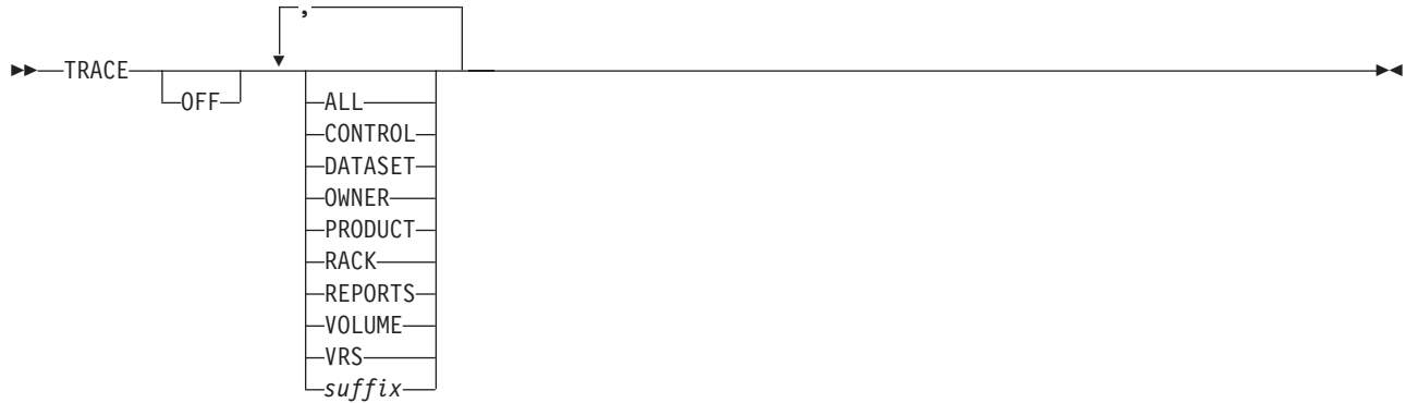
Figure 4. TRACE command syntax diagram
