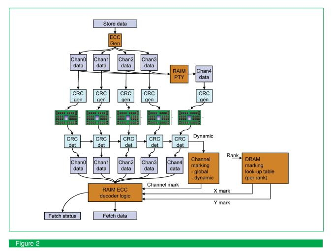
RAIM ECC design static channel and DRAM marking and dynamic CRC marking. (gen: generation; det: detection; PTY: parity.)
