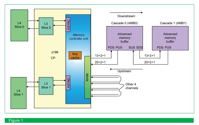
zEnterprise memory subsystem. Two-cascade example (one channel shown). (CP: central processor; RAIM: redundant array of independent memory; PDS: primary downstream receiver; SDS: secondary downstream driver; PUS: primary upstream driver; SUS: secondary upstream receiver; AMB0: advanced memory buffer on cascade 0; AMB1: advanced memory buffer on cascade 1.)
