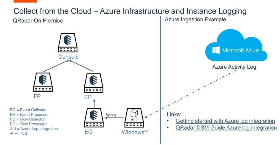
This diagram outlines how event collection works for Azure Activity Logs today. Data is sent to the Azure Log Integrator and queried by the QRadar On Premise appliance using a REST API. \*\* The Azure log integration service can be on premise or in the Azure Cloud (See Getting Started)
