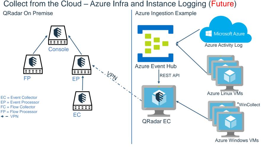
This diagram outlines an architecture concept for hosting a QRadar Event Collector in the Azure Cloud.
