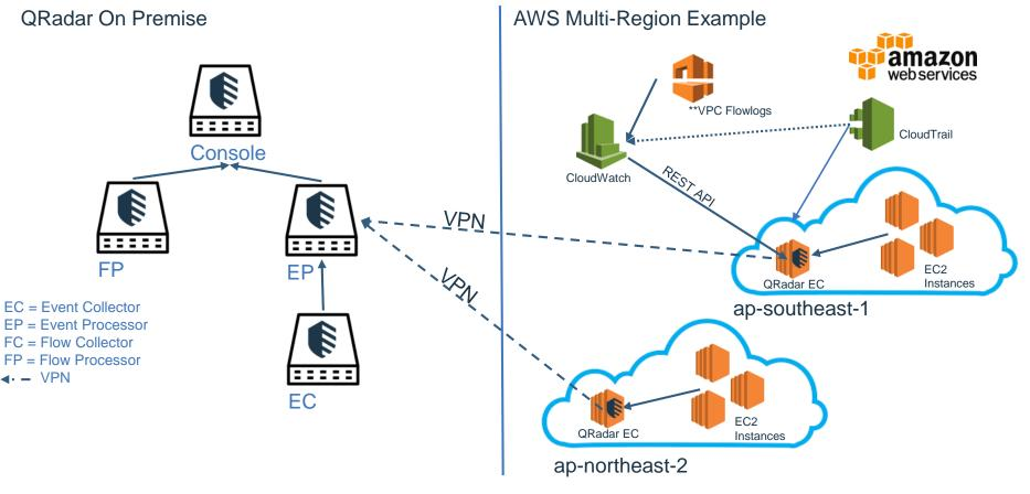
This diagram outlines collection with an Event Collector in the Cloud. Data is collected on the Cloud EC and the QRadar pipeline sends the data to an EP On Premise appliance. A benefit is that you save on bandwidth as the event pipeline compresses EC to EP connections. Searches are completed with the on premise appliances.
