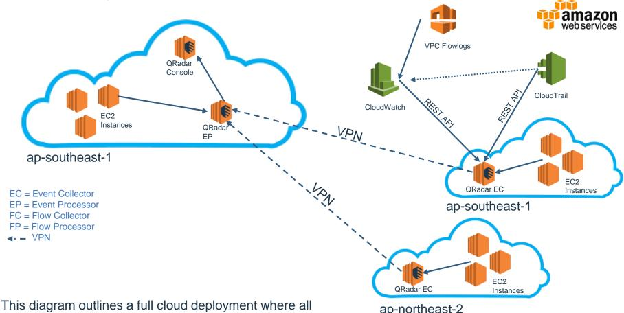
appliances are installed in the AWS Cloud.
