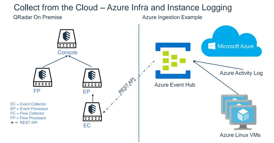
This diagram outlines how event collection works for the Azure Event Hub. Data is sent to the Azure Event Hub and queried by the QRadar On Premise appliance using a REST API.
