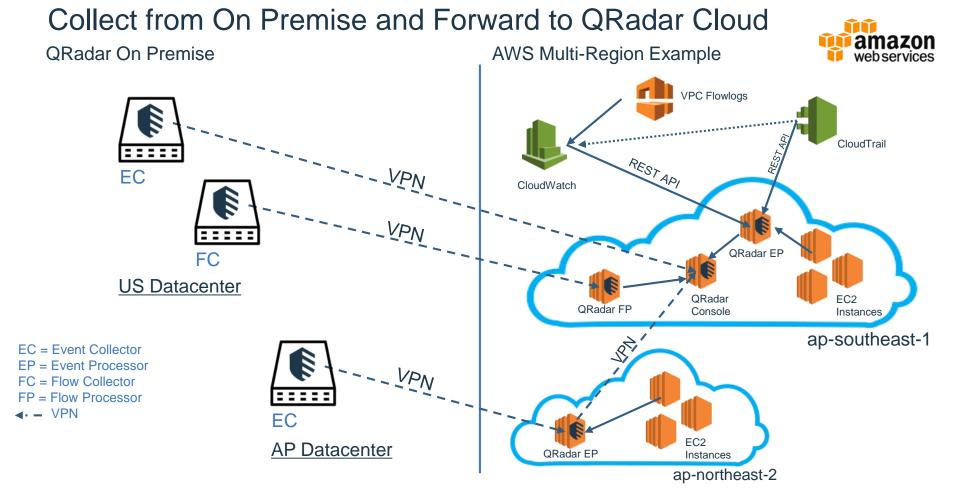
This example outlines on premise Event Collector and Flow Collector appliances that VPN data to the QRadar Cloud deployment. A benefit here is it limits the requirement for HA due to Cloud resiliency.
