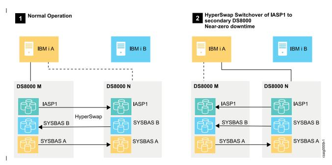
The above diagram represents a combination HyperSwap plus LUN switching environment. If the production DS8000 has a planned outage, a HyperSwap switch can be initiated to the target DS8000 with near zero downtime. This type of switch does not involve switching access of the IASP from IBM i A to IBM i B or a vary off and vary on of the IASP.
