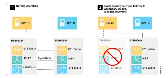
The above diagram represents a combination HyperSwap plus LUN switching environment. If the production DS8000 has an unplanned outage, a HyperSwap failover is automatically initiated to the target DS8000 with minimal downtime (seconds to minutes). This type of switch does not involve switching access of the IASP from IBM i A to IBM i B or a vary off and vary on of the IASP.
