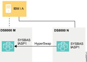
Since HyperSwap uses DS8000 Metro Mirror function, data transfer is done synchronously. You must be aware of the same distance limitations, and bandwidth requirements that are associated with transmission times as with any solution when synchronous communications are sent.
