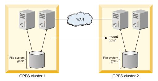
Figure 2. A multicluster configuration
