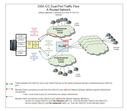
Figure 46. Network topology Diagram 2
