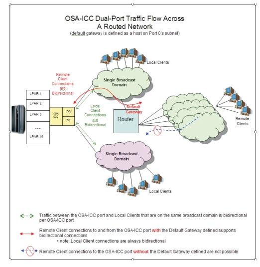
Figure 1. Network topology diagram
