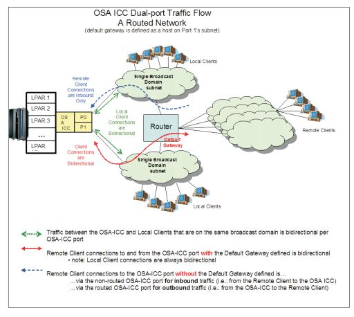
Figure 47. Network topology Diagram 3
