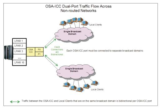
Figure 45. Network topology Diagram 1
