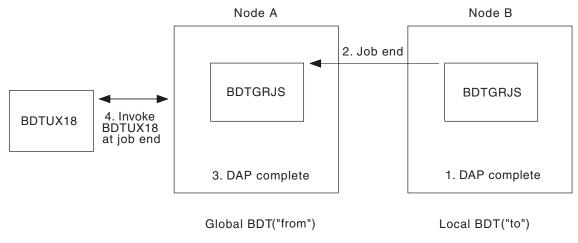
Figure 35. Flow diagram for the invocation of BDTUX18 (job end)
