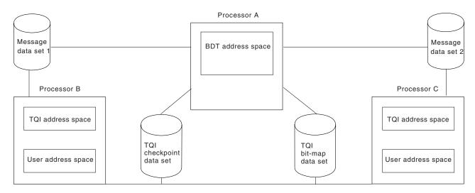
Figure 4. Example of TQI in a three-processor JES complex
