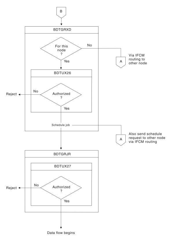
Figure 29. Routing of a file-to-file transaction
