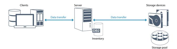
Figure 1. Components in the Tivoli Storage Manager data protection solution
