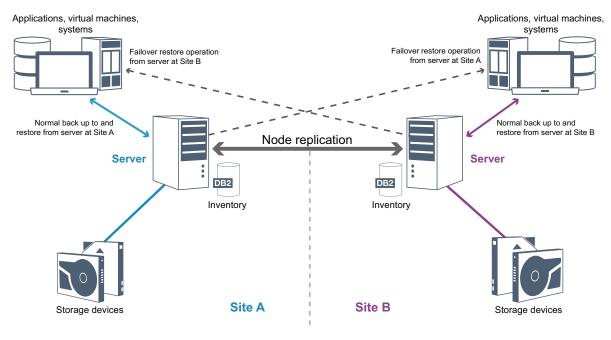
Figure 13. Automatic failover process
