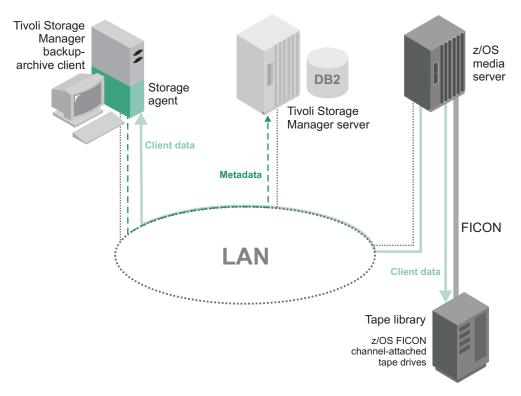
Figure 3. Data movement in a z/OS media server environment. Solid lines indicate data movement. Solid lines with arrows indicate client data. Broken lines indicate movement of control information and metadata.
