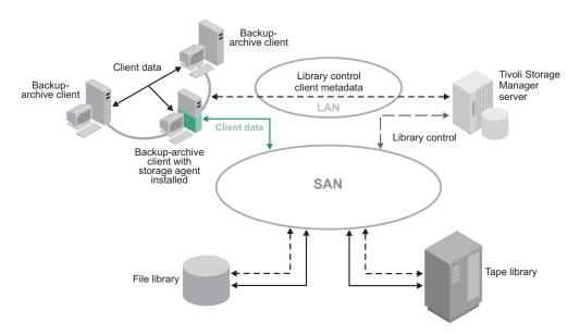
Figure 2. SAN data movement with the LANFREECOMMMETHOD option. Solid lines indicate data movement. Broken lines indicate movement of control information and metadata.
