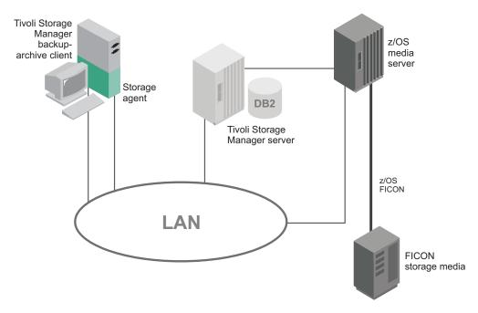
Figure 11. Network connection between a storage agent, a Tivoli Storage Manager server, and a z/OS media server. Client data is transferred between the storage agent and the z/OS media server.
