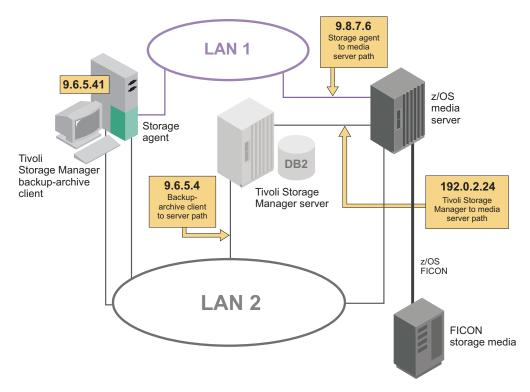
Figure 12. Network connection between a storage agent, a Tivoli Storage Manager server, and a z/OS media server, using two LANs.
