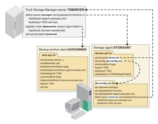
Figure 4. Connections between the client, storage agent, and server. The passwords are shown as xxxxxxx because they are encrypted in the file.
