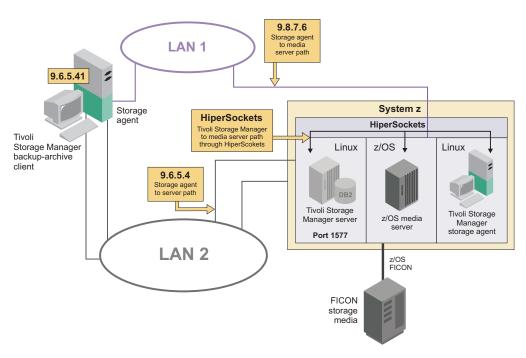
Figure 13. Data movement from a storage agent to a Linux for System z can communicate with a z/OS media server using HiperSockets.
