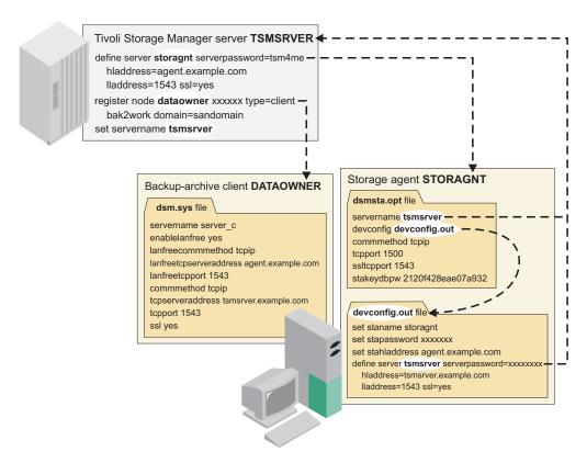
Figure 3. Connections between the client, storage agent, and server. The passwords are shown as xxxxxxx because they are encrypted in the file.
