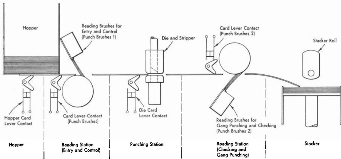
Figure 12. Schematic of Read and Punch Unit
