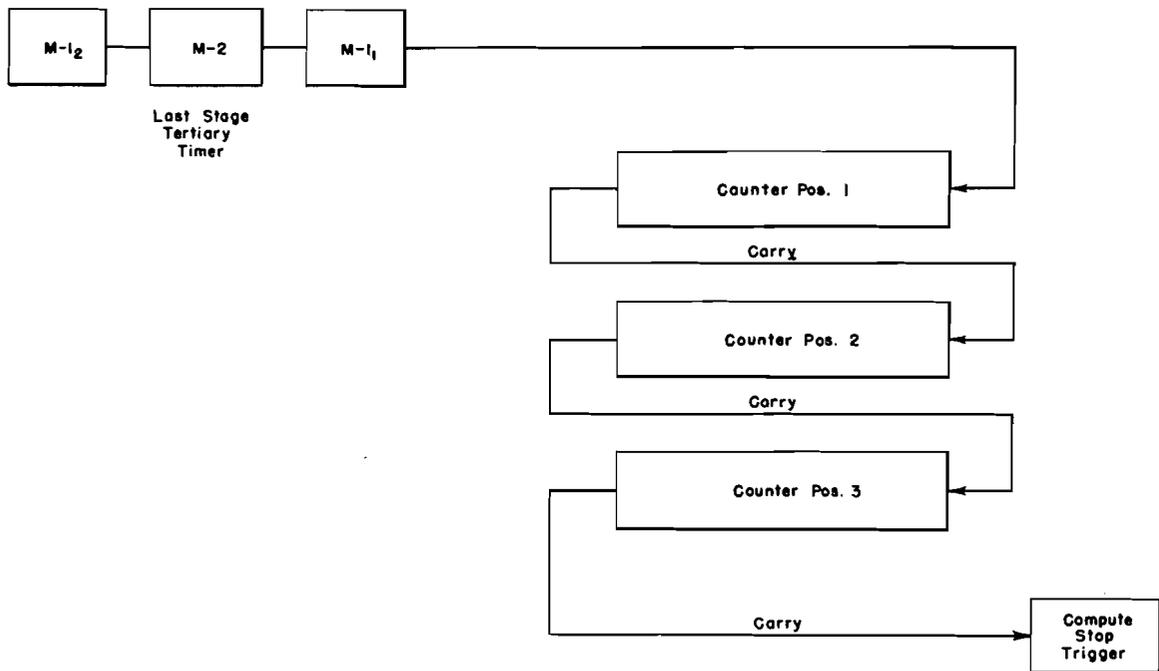
Figure 130. Connections for Manual Checking of Multivibrator Frequency
