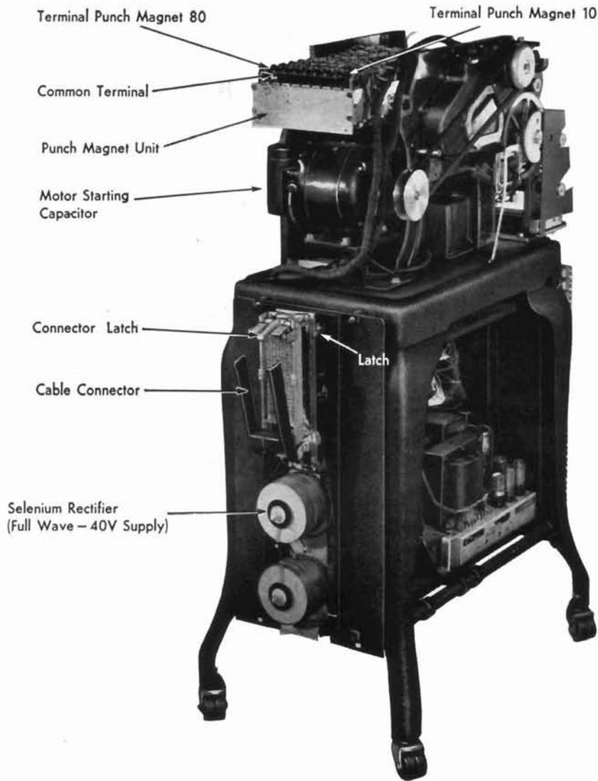
Figure 8. Read and Punch Unit—Right Side View
