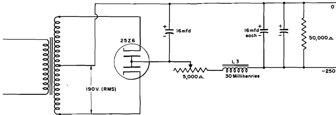
Figure 55. Schematic of -250 Volt Rectifier Circuit
