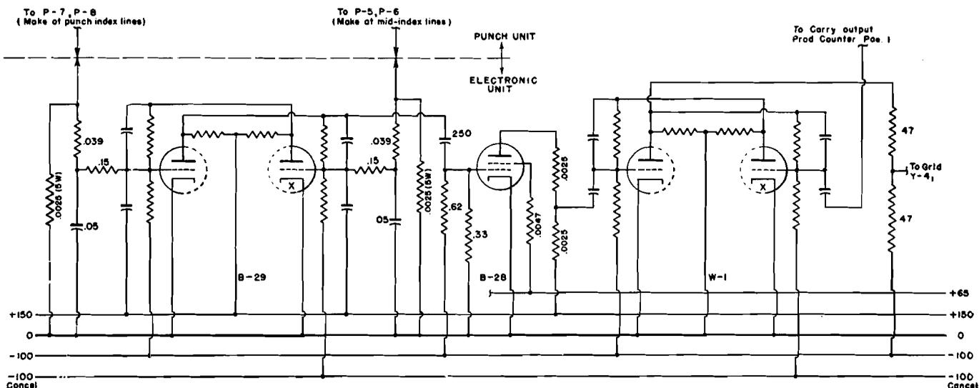
Figure 129. Triggering Off of Read-out Triggers at Mid-Index
