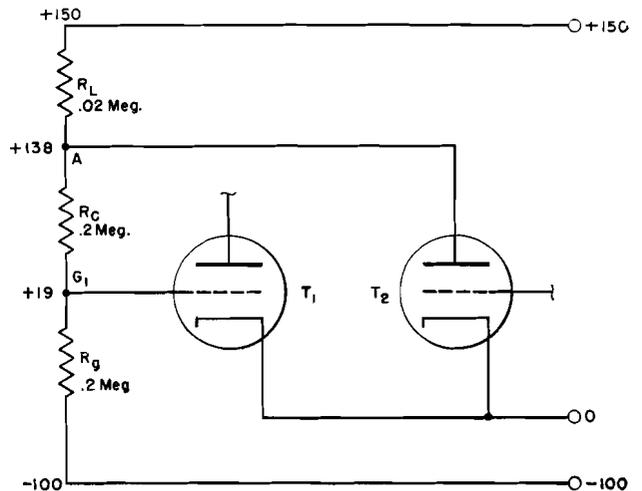
Figure 75. Anode of T<sub>2</sub> Controls Grid of T
