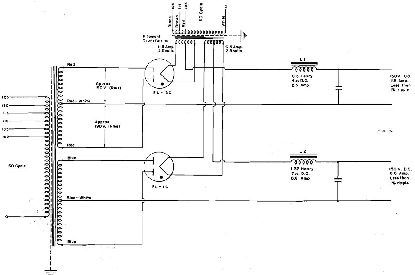
Figure 54. Tube Power Supply Transformers, Rectifiers, and Chokes
