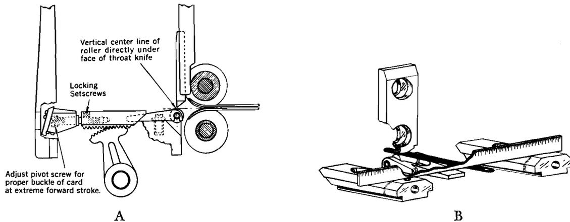
Figure 35. Feed Adjustments
