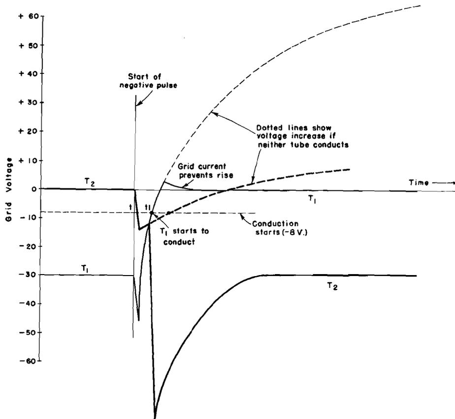
Figure 80. Oscillogram of Actual Grid Voltages During Triggering
