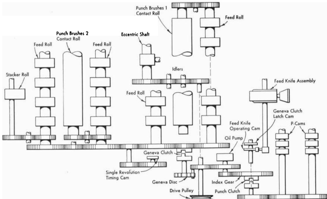
Figure 16. Schematic of Drive Mechanism
