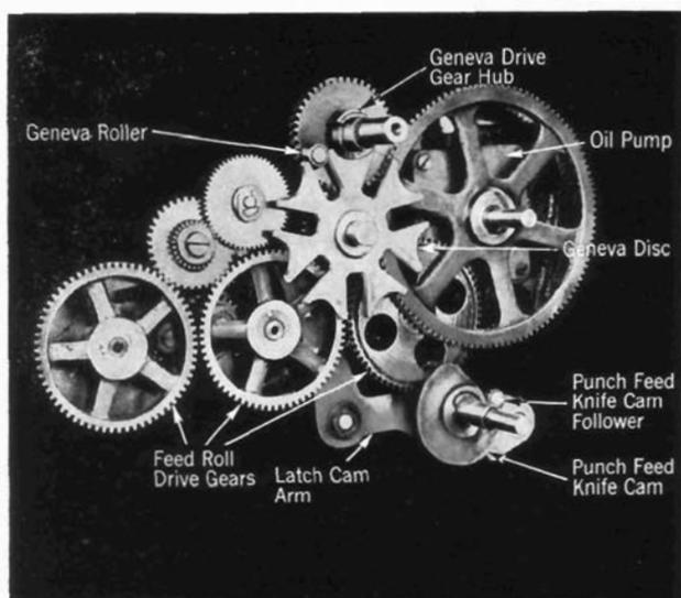
Figure 19. Geneva Mechanism
