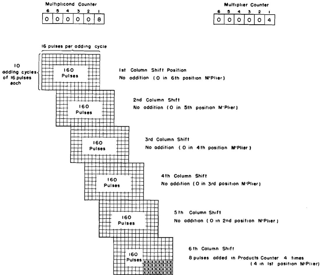
Figure 60. Block Diagram of Multiplication by Over-and-Over Addition
