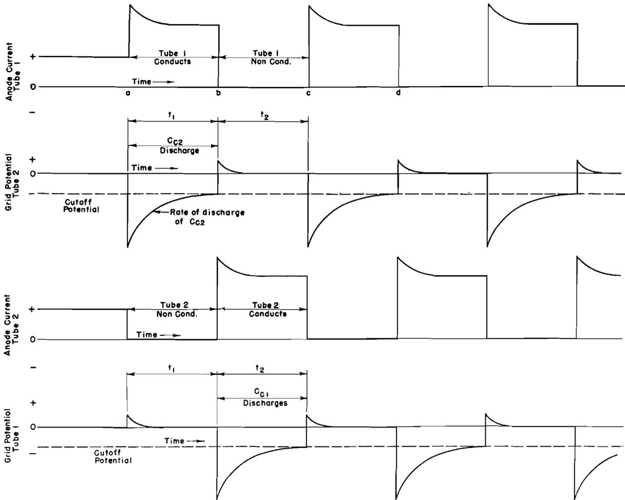
Figure 101. Voltage and Current Curves for Multivibrator
