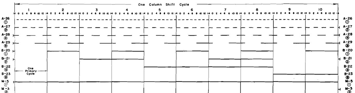
Figure 108. Relationship Between Primary and Secondary Timers
