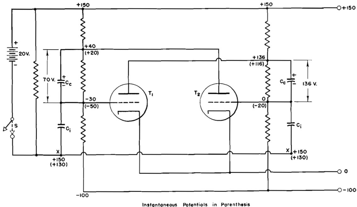
Figure 77. Use of Capacitors in Trigger Circuit
