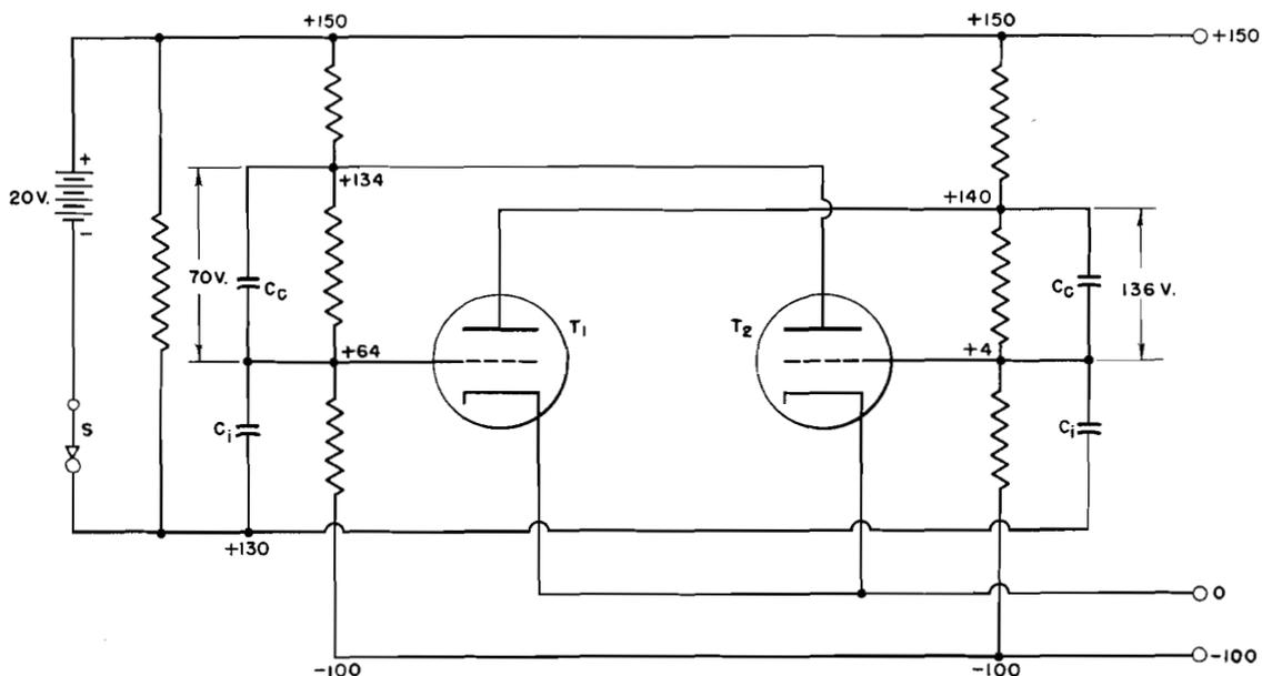
Figure 78. Voltages Existing after C<sub>i</sub> Discharges but before C<sub>c</sub> Discharges with Neither Tube Conducting
