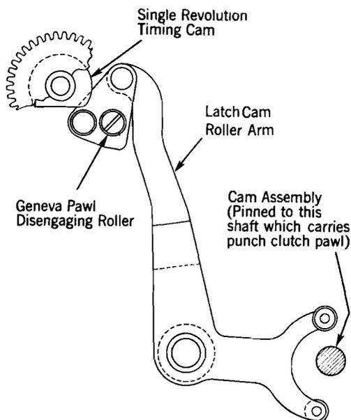
Figure 22. Single Revolution Timing Cam
