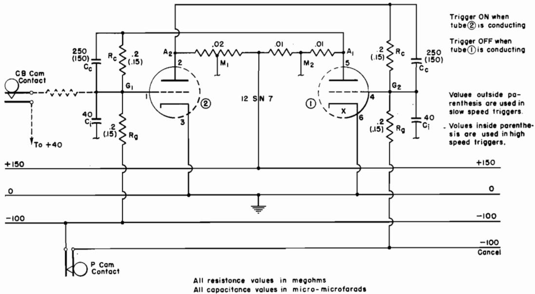
Figure 85. Actual Trigger Circuit Used in Type 603
