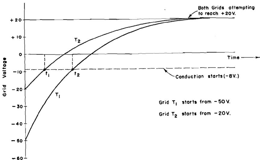
Figure 83. Rise in Grid Voltage as Capacitors Discharge
