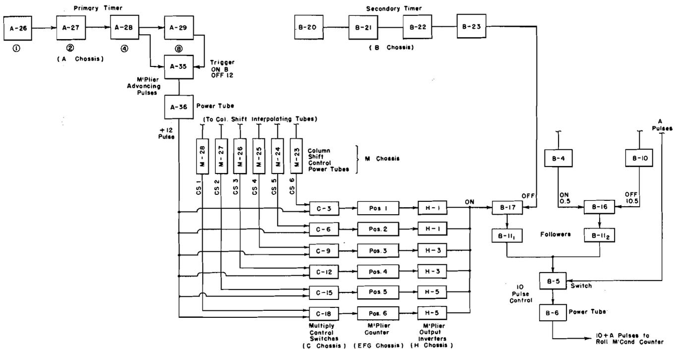
Figure 111. Block Diagram of Multiplier Advancing Circuits
