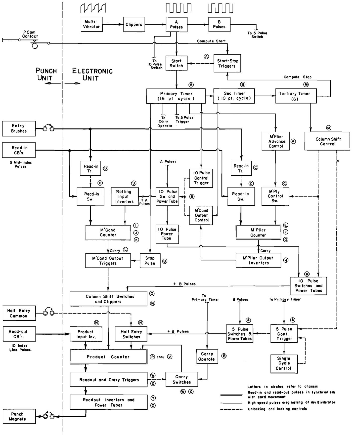
Figure 64. Block Diagram of Type 603 Circuits
