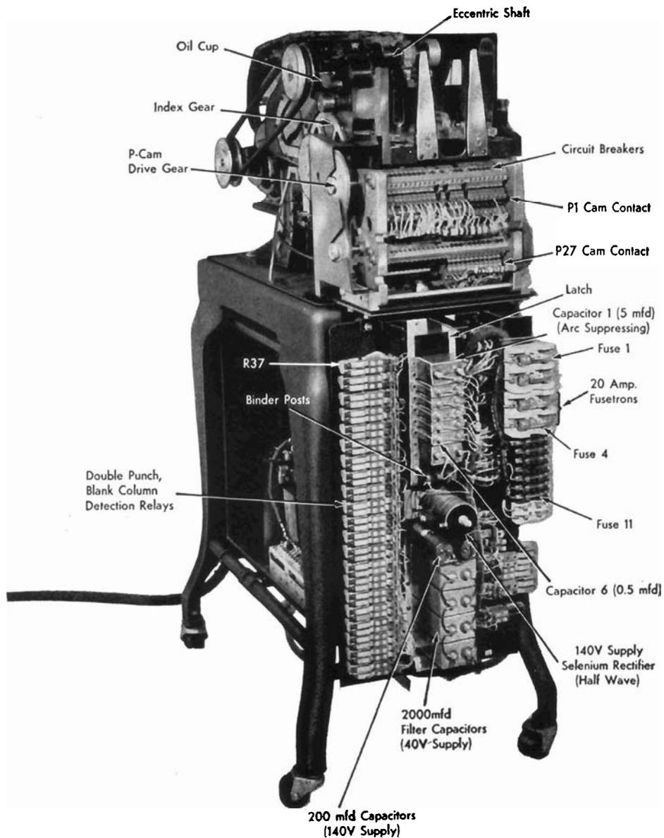
Figure 9. Read and Punch Unit—Left Side View
