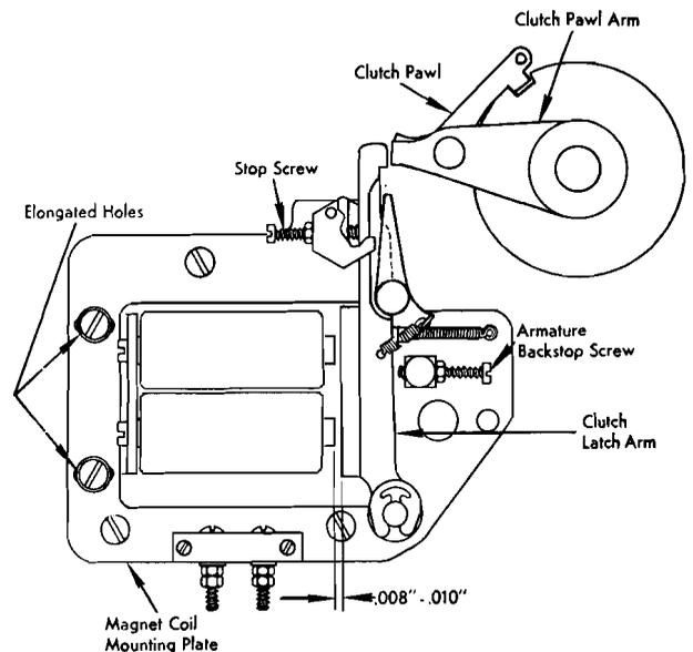
Figure 31. Clutch Adjustment
