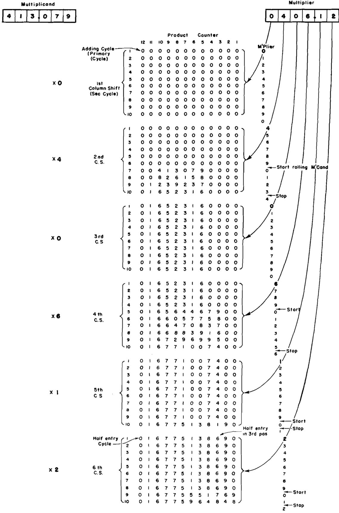
Figure 61. Principle of Multiplication Showing Detailed Operation
