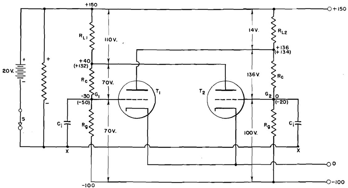
Figure 82. Application of Pulse to Trigger Circuit Without Cc Capacitors
