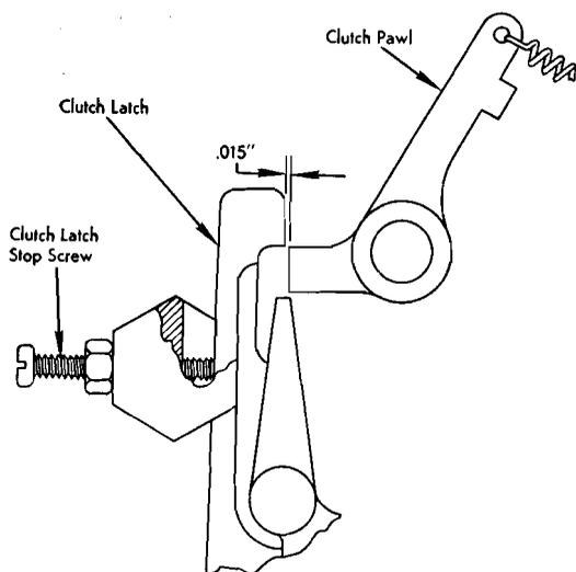
Figure 29. Clutch Adjustment
