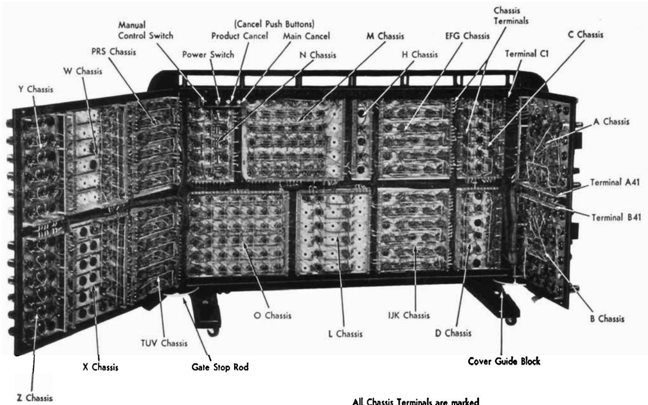
Figure 15. Electronic Computing Unit with Gates Open
