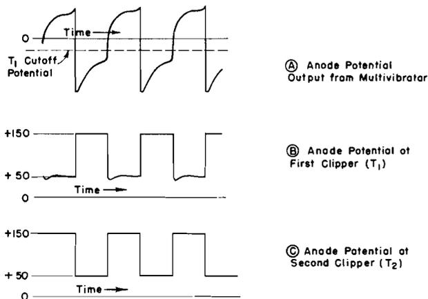
Figure 104. Output Voltages of Multivibrator and Triode Clippers
