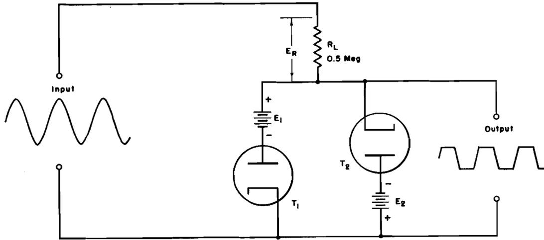
(A) Diode Peak Clipping Circuit
