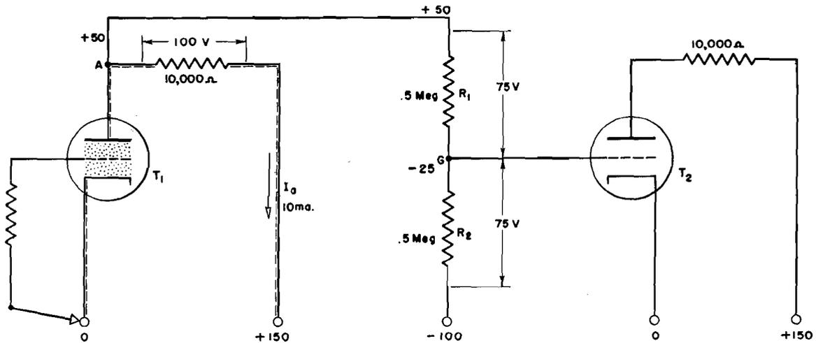
Figure 69. Direct-Coupled Triodes
