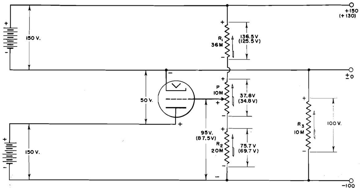
Figure 56. Schematic of Voltage Ratio Regulator Circuit
