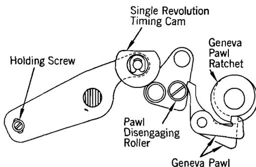
Figure 33. Single Revolution Timing Cam and Bracket Adjustment
