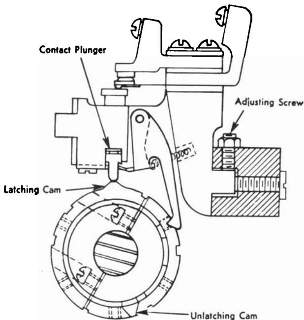
Figure 28. Contact Cam
