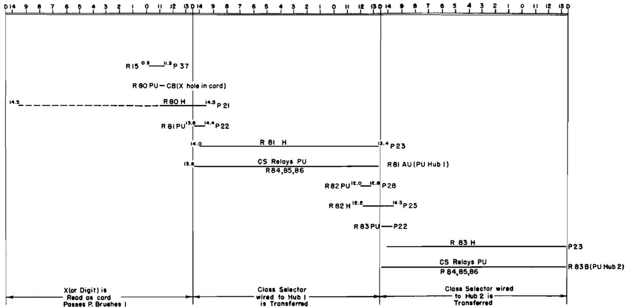
Figure 52. Sequence of Operation of Class Selectors
