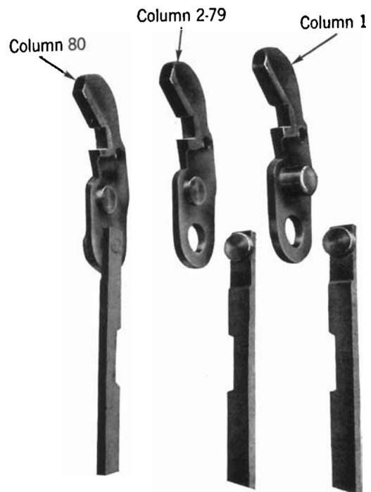
Figure 25. Three Types of Interposers
