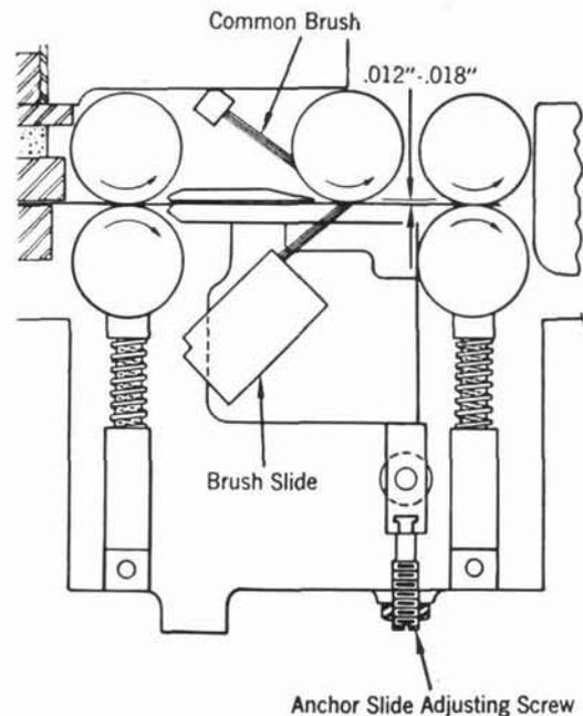
Figure 39. Anchor Slide Adjustment
