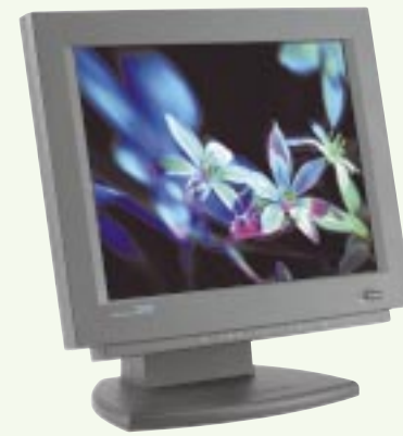
IBM's flat-panel displays are one-sixth the depth and 85% of the width/height of the equivalent cathode ray tube (CRT) products. They use 50% - 66% less energy and generate less than one-third the heat of the equivalent CRT.
